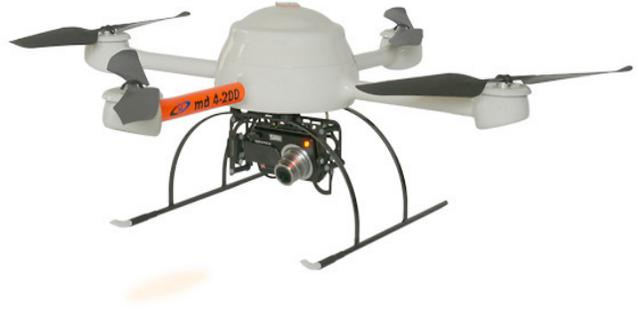
Fig. 2. A quad-rotor microdrone model md4-200
