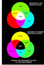
FIGURE 6.6 Primary and secondary colors of light and pigments. (Courtesy of the General Electric Co., Lamp/Business Division.)
