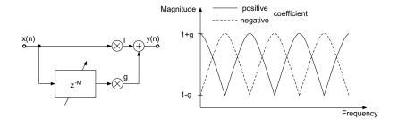
Mix input with a delayed version of filter output:
