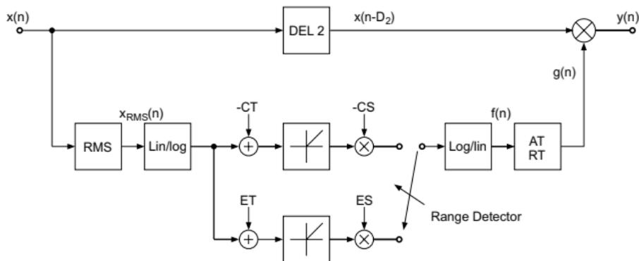
Noise gate Attenuate signal if level is below threshold
