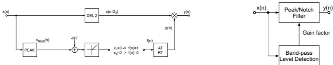
De-esser control notch gain using BPF level measurement (2-6 kHz)
