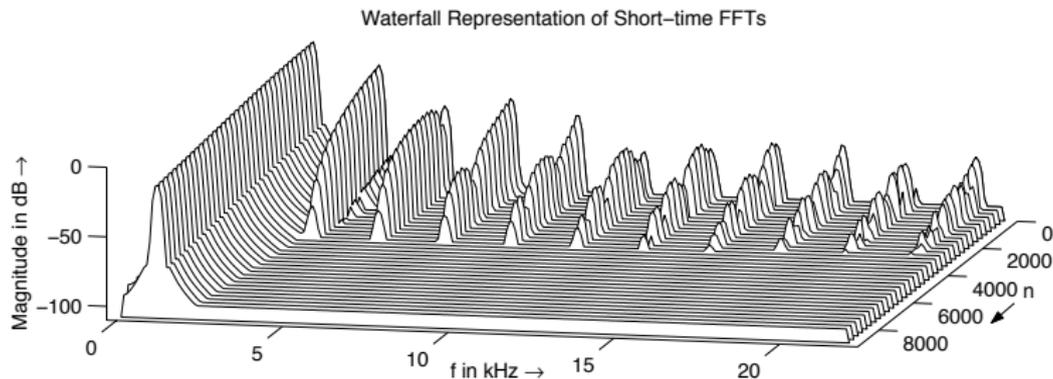
Adds odd harmonics, decay with increasing frequency
