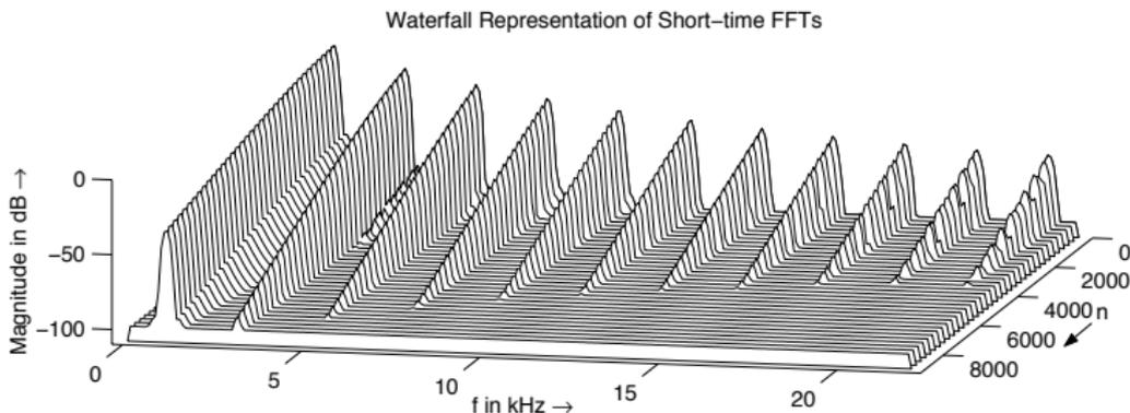
Adds odd harmonics, decay with increasing frequency
