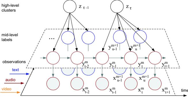
**Fig. 1.** The layered dynamic mixture model, in the dimensions of time, various modalities and perceptual levels. Shaded nodes: observed, clear nodes: hidden; different colors represent nodes in different modality.
