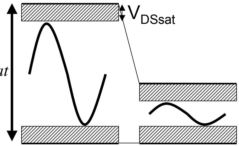
$$\text{Penalty factor} = 1 + \frac{2V_{DSsat}}{(V_{DD} - 2V_{DSsat})}$$
