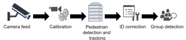
Figure 2: Different stages in the Auto-SDA pipeline.
