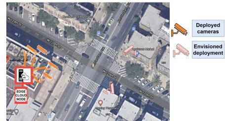
Figure 1: The NSF PAWR COSMOS pilot site at 120 th St. and Amsterdam Ave. intersection, NYC. Cameras are deployed on the Columbia University's Mudd building and connected to the edge-cloud servers via dedicated fibers.
