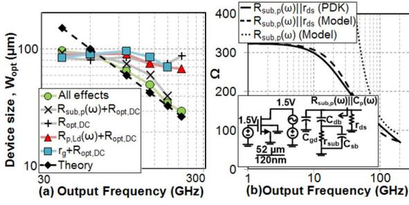
Fig. 3. (a) Device size needed to deliver maximum power to a  $50 \Omega$  load in a 130 nm CMOS balanced doubler. (b) Frequency dependence of  $R_{\text{sub},p}$ .
