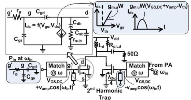
Fig. 2. Circuit diagram of a simple balanced CMOS frequency doubler.
