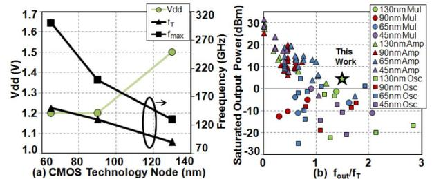
Fig. 1. (a) Scaling of supply voltage and cutoff frequency ( $f_T$ ) across CMOS nodes. (b) Comparison of this work with state-of-the-art CMOS sources across output frequency normalized to technology  $f_T$ .
