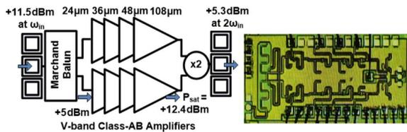
Fig. 6. Block diagram and chip photo of the 130 nm CMOS F-band doubler. The annotated values are at 67 GHz after post-layout simulations.
