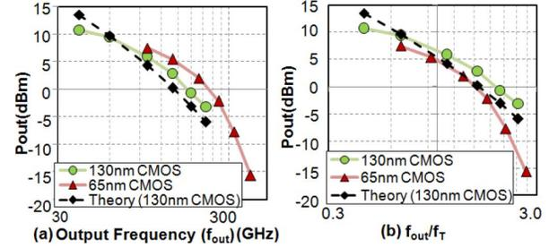
Fig. 5. Simulated output power for optimal doublers driving  $50 \Omega$  in 130 nm and 65 nm CMOS across (a) absolute  $f_{\text{out}}$ , (b)  $f_{\text{out}}$  normalized to  $f_T$ .
