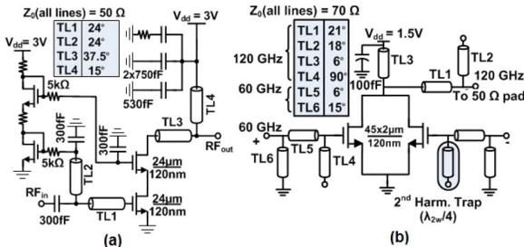
Fig. 7. (a) First V-band amplifier stage and, (b) the F-band balanced doubler.
