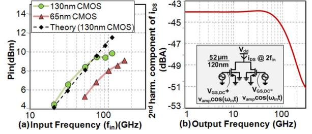
Fig. 4. (a)  $P_{\text{in}}$  of optimal doubler driving  $50 \Omega$  across frequency. (b) Frequency dependence of 2nd harmonic current due to NQS effect in 130 nm.
