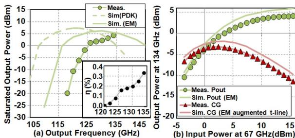
Fig. 8. (a) Measured and simulated saturated output power and efficiency. (b) Output power and conversion gain at 134 GHz.
