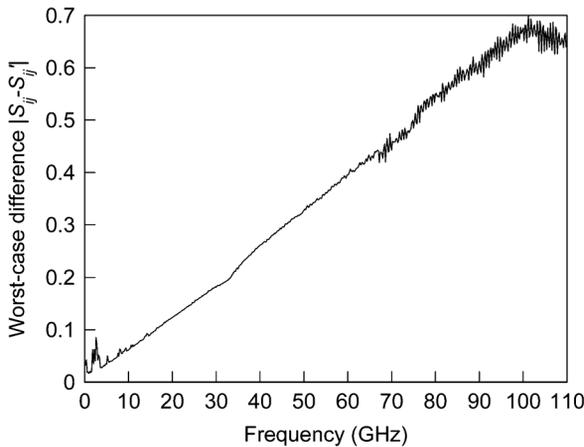
Fig. 3. Worst case differences between measurements corrected by the TRL and SOLT calibrations.
