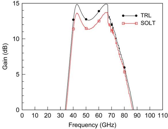
Fig. 2. Comparison of amplifier gain corrected with TRL and SOLT. We used the maximum power available from our VNA to try to maximize the power generated by the amplifier. An increase in power level in the VNA at 67 GHz caused the drop in gain seen above.
