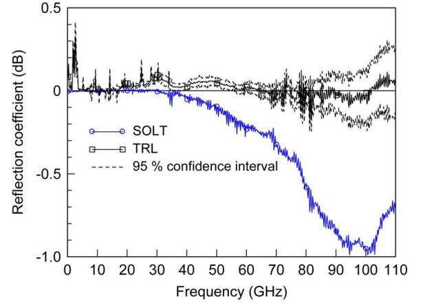
Fig. 4. Open pad corrected by the SOLT and TRL calibrations.
