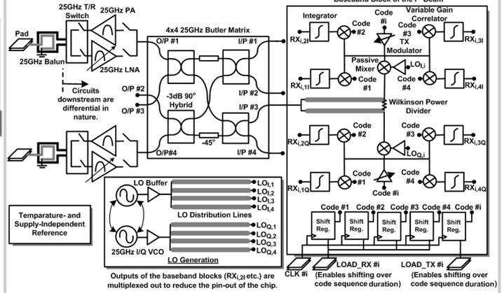
Figure 11.1.2: Block diagram of the 90nm CMOS, 4-channel, 4-beam, 24-26GHz, Spatio-Temporal RAKE radar transceiver.
