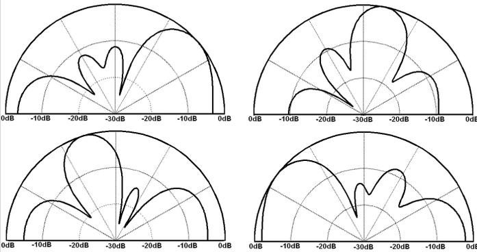
Figure 11.1.3: Synthesized normalized array patterns for the 4x4 Butler matrix based on measured S-parameter data.
