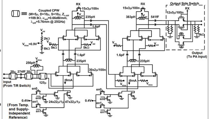
Figure 11.1.4: Schematic of the 90nm CMOS, 25GHz, front-end LNA.
