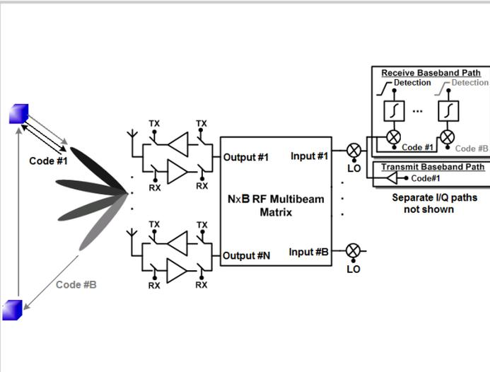
Figure 11.1.1: Spatio-Temporal RAKE radar concept.
