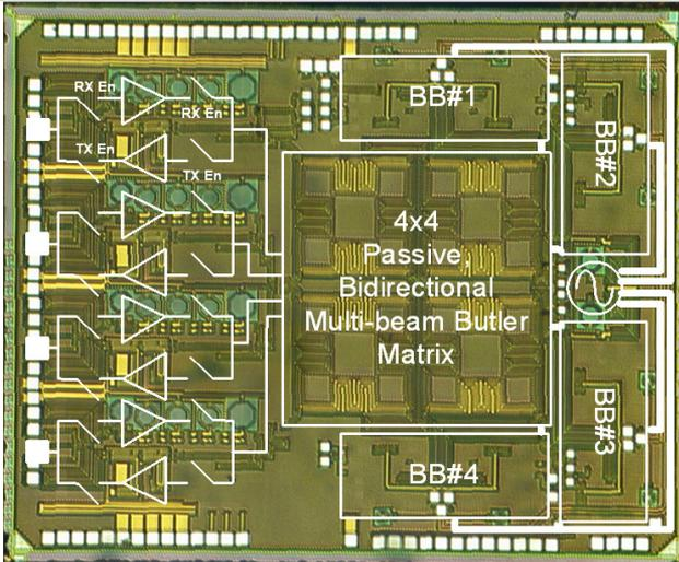
Figure 11.1.7: Chip micrograph of the 90nm CMOS, 4-channel, 4-beam, 24-26GHz, Spatio-Temporal RAKE radar transceiver. The radar chip consumes an area of 3.4mm $\times$ 4.2mm.
