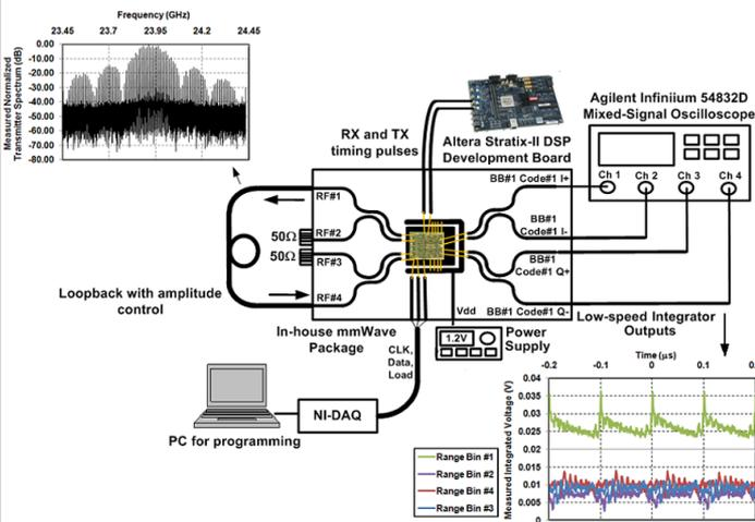
Figure 11.1.5: Wired loopback radar testing.
