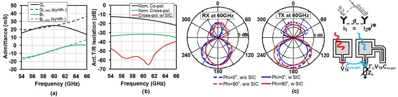
Fig. 4. Simulations of the antenna cancellation: (a) required and synthesized reflective termination admittance, (b) resultant antenna cancellation, and (c) effect of SIC on the RX and TX radiation patterns.
