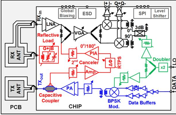
Fig. 2. Architecture of the full-duplex 60GHz TRX with reconfigurable polarization-based antenna and RF cancellation.
