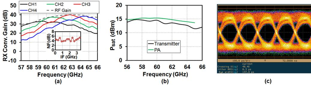
Fig. 6. (a) RX conversion gain in all 4 IEEE channels at highest gain setting, RF gain across frequency (swept RF and LO with fixed 120 MHz IF), and NF in channel 3. (b) PA and TX saturated output power versus frequency. (c) TX-RX 5Gbps BPSK loopback test.
