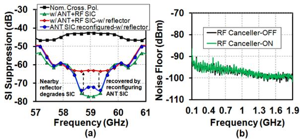
Fig. 7. (a) Measured SI suppression across frequency with antenna and RF cancellation configured. Bringing a reflector 1.5cm away from the antennas degrades the SI suppression, but it can be recovered by reconfiguring the antenna cancellation. (b) RF canceller's effect on the receiver output noise (RBW=51kHz).
