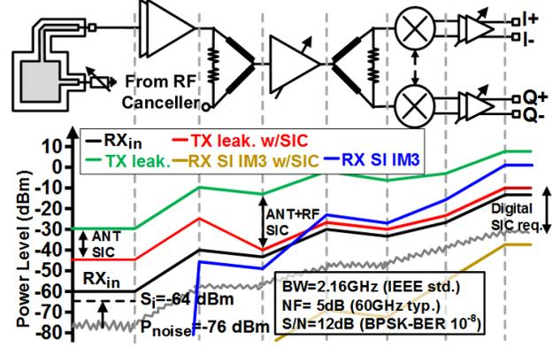
Fig. 3. Received signal, SI, RX noise floor and SI IM3 products generated in the RX (with and w/o SIC) through the chain.
