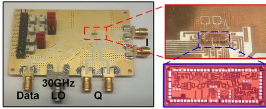
Fig. 5. PCB, antennas and chip photo of the 1.3mm x 3.4mm IC.
