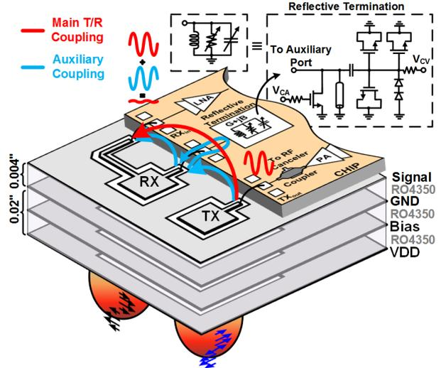
Fig. 1. Proposed polarization-based reconfigurable wideband self-interference cancellation concept.
