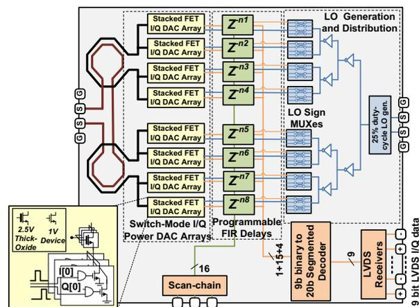
Fig. 1: Architecture of the proposed RF I/Q Power DAC transmitter with integrated quantization noise filtering.
