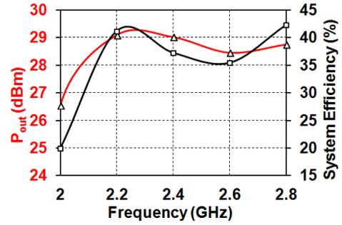
Fig. 5: Peak output power and efficiency across frequency of the transmitter. Main  $V_{dd} = 2.6V$ , Driver  $V_{dd} = 1.2V$
