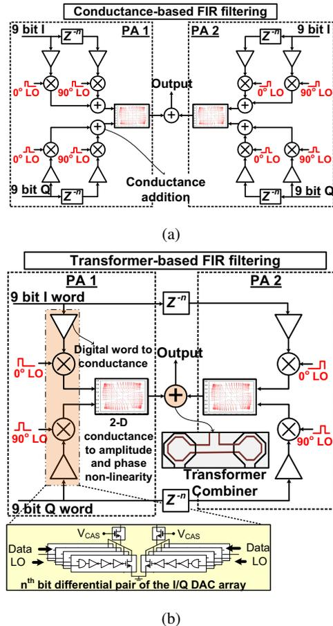
Fig. 2: Configuration for FIR filtering through (a) addition of device conductances and (b) the proposed transformer-based FIR filtering with addition across the transformer.
