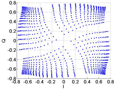
Fig. 7: The two dimensional nonlinearity constellation obtained for equally spaced values of I and Q. Only  $32 \times 32$  points are shown here.
