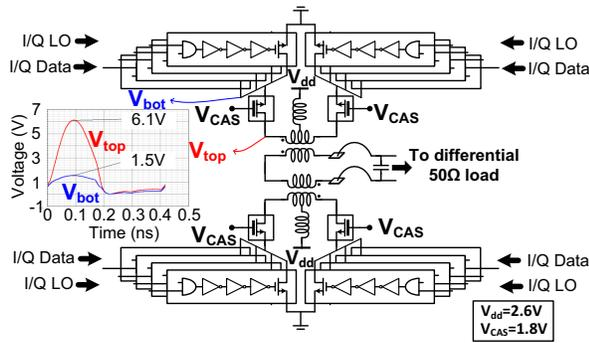
Fig. 3: Circuit diagram of the transformer combined Class E/ $F_{odd}$  digital PAs.
