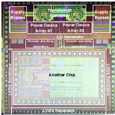
Fig. 4: Chip photograph of the transmitter.
