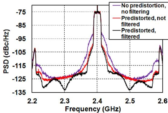
Fig. 8: PSD of the output of the transmitter normalized to total signal power showing the effect of 2D I/Q DPD and third-order two-tap transformer-based FIR filtering.
