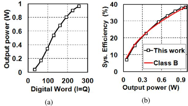
Fig. 6: (a) Output power vs. DCW for  $I=Q$  and (b) resultant system efficiency under back-off at 2.4 GHz. Main PA  $V_{dd} = 2.8V$ , Driver PA  $V_{dd} = 1.3V$ .
