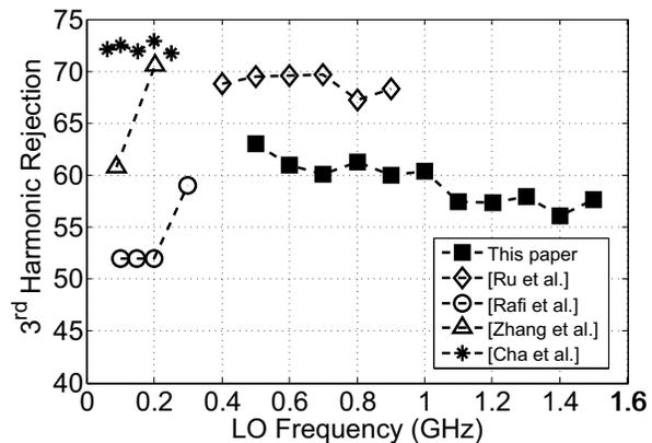
Fig. 8. A comparison for the 3<sup>rd</sup> harmonic rejection at various LO frequencies with the state-of-the-art HRMs.
