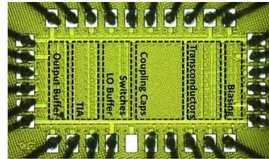
Fig. 6. Die photo of the prototype chip.
