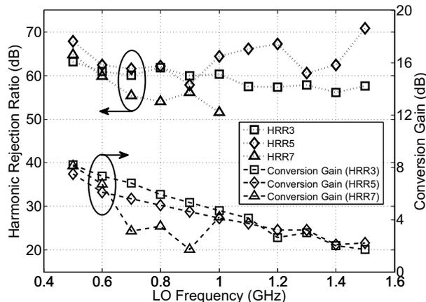
Fig. 7. Measured 3<sup>rd</sup>, 5<sup>th</sup> and 7<sup>th</sup> harmonic rejection and the corresponding conversion gain of the mixer for various LO frequencies.
