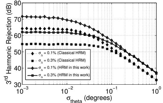
Fig. 3. Theoretically achievable 3<sup>rd</sup> harmonic rejection in the presence of gain and phase mismatches for the proposed HRM architecture and the classical HRM.
