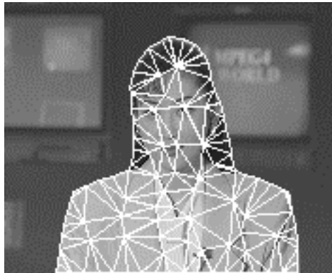
Figure 9- 2D mesh modeling of the "Akiyo" video object
