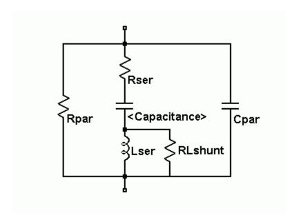
Capacitor Instance Parameters
