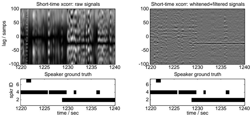
**Fig. 2.** Short-time cross-correlations on raw signals (left panel) and after LPC whitening and filtering (right panel). Vertical axis is lag; horizontal axis is time; darker pixels indicate higher normalized cross-correlation. The ground-truth speaker labels are shown below each pane; there is a visible transition between speaker 2 and speaker 4 around  $t = 1229$  sec.
