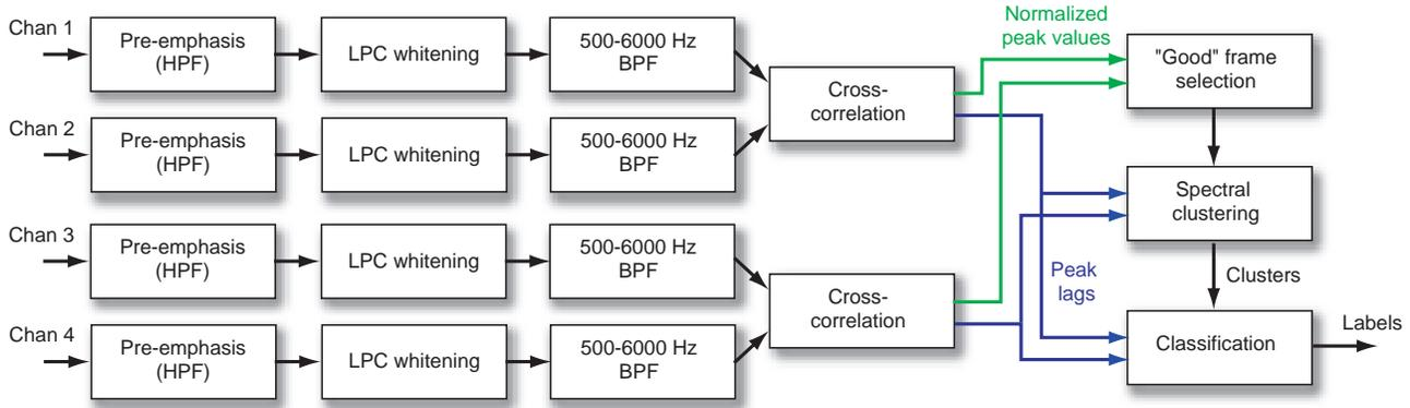
Fig. 1. Overview of the timing difference classification system.
