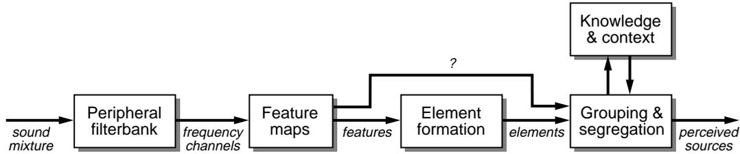
Figure 1: Block-diagram of the possible structure auditory organization, as typically assumed by modellers. The bypass around “element formation” acknowledges the debate over whether segmentation can be done in a purely bottom-up fashion, or whether it must depend on top-down knowledge.
