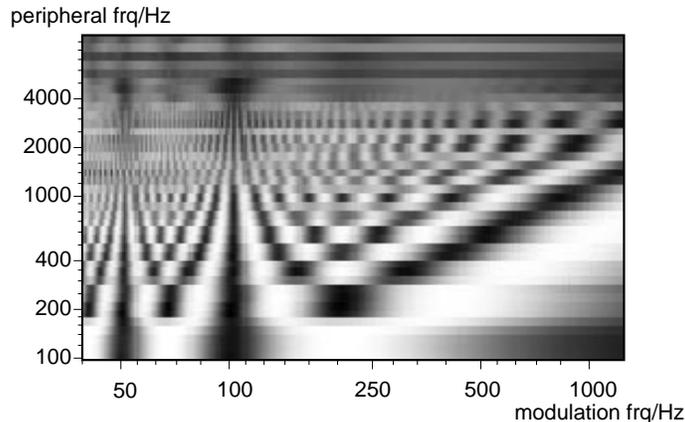
Figure 3: An example of a peripheral frequency/modulation frequency display, showing typical features for a periodic signal. Both axes are logarithmic. Because this example is autocorrelation-based, it displays subharmonics (e.g. the ridge at 50 Hz for this 100 Hz signal; a display based on band-pass filters would instead show modulation overtones or superharmonics, e.g. at 200 Hz).
