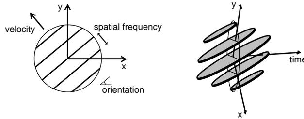
Figure 2: The three-dimensional kernels of Heeger (1987) are sensitive to grids with a particular spacing and orientation, moving in the image plane at a particular velocity.
