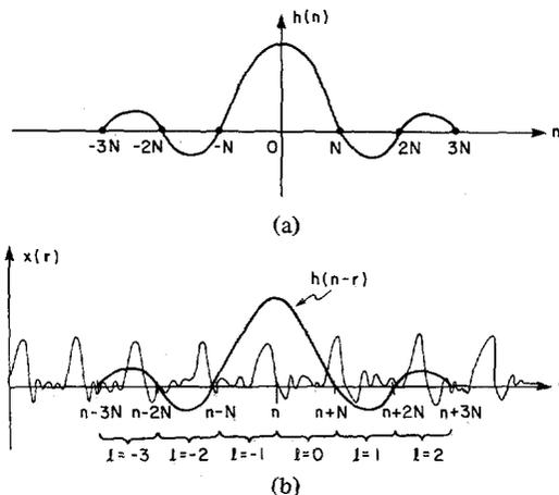
Fig. 3. (a) Typical unit-sample response for prototype low-pass filter  $h(n)$ . (b)  $h(n)$  shifted and superimposed on input sequence  $x(r)$ .
