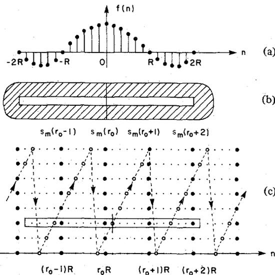
Fig. 6. (a) Typical unit-sample response for  $1:R$  FIR digital interpolating filter. (b) Mask to extract values required for interpolation using  $f(n)$ . (c) Net associated with  $x_m(n)$ . • indicates points representing  $s_m(r) = x_m(rR)$ . ○ indicates points representing  $x(n) = x_m(n)$ .
