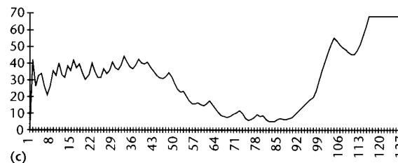
Figure 11. Psychoacoustic model 1 processing. (a) Identified tonal and nontonal components. (b) Decimated tonal and nontonal components. (c) Global masking thresholds.
