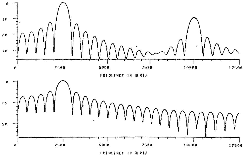
FIGURE 29. This is the result of approximating the Fourier integral by Simpson's composit rule. An effective halving of the sampling rate and corresponding aliasing occurs. The lower plot approximates the integral by the triangle rule with somewhat better success.
