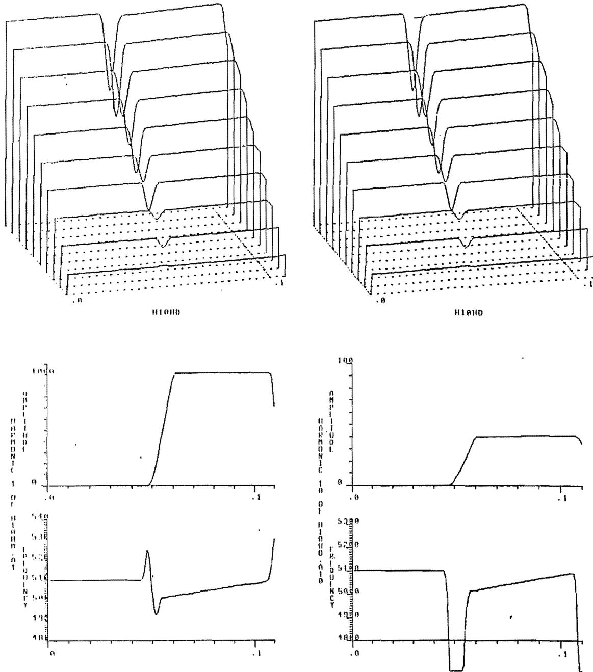
FIGURE A7. This shows the output of the heterodyne filter for a synthesized input signal which consists of a 500 Hz signal with a 10 millisecond linear attack on each harmonic. Each harmonic is 70% of the amplitude of the previous harmonic. Here we slew the frequency of the note from 500 Hz to 505 Hz over the duration of the tone. This is a 1% change, less than a quarter-step. Even in this case, the heterodyne filter seems to track acceptably.
