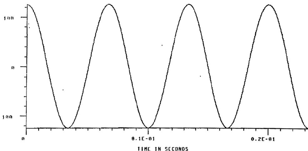
FIGURE 4. This is the autocorrelation of a pure sinusoid. The result is, as we would expect, a pure sinusoid with a maximum at integral multiples of the period.
