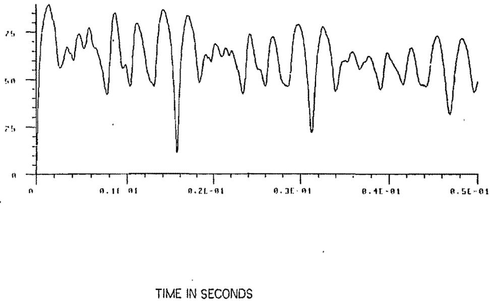
FIGURE 15. Equation (18) applied to C-major chord in root position. The notes in the chord are C4, E4, and G4. We see a distinct minimum at 15.5 milliseconds, which is C2.
