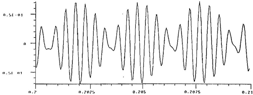
FIGURE 1. This waveform was produced by filtering the waveform of a guitar tone so as to select only a few of the upper harmonics. The note that was being played was roughly an E4 (332 Hz). The sixth and seventh harmonics were most prominent in this waveform, although many others are present to a lesser extent. It is clear that the waveform is periodic with a period of roughly 3 milliseconds, which corresponds to the frequency of the note.
