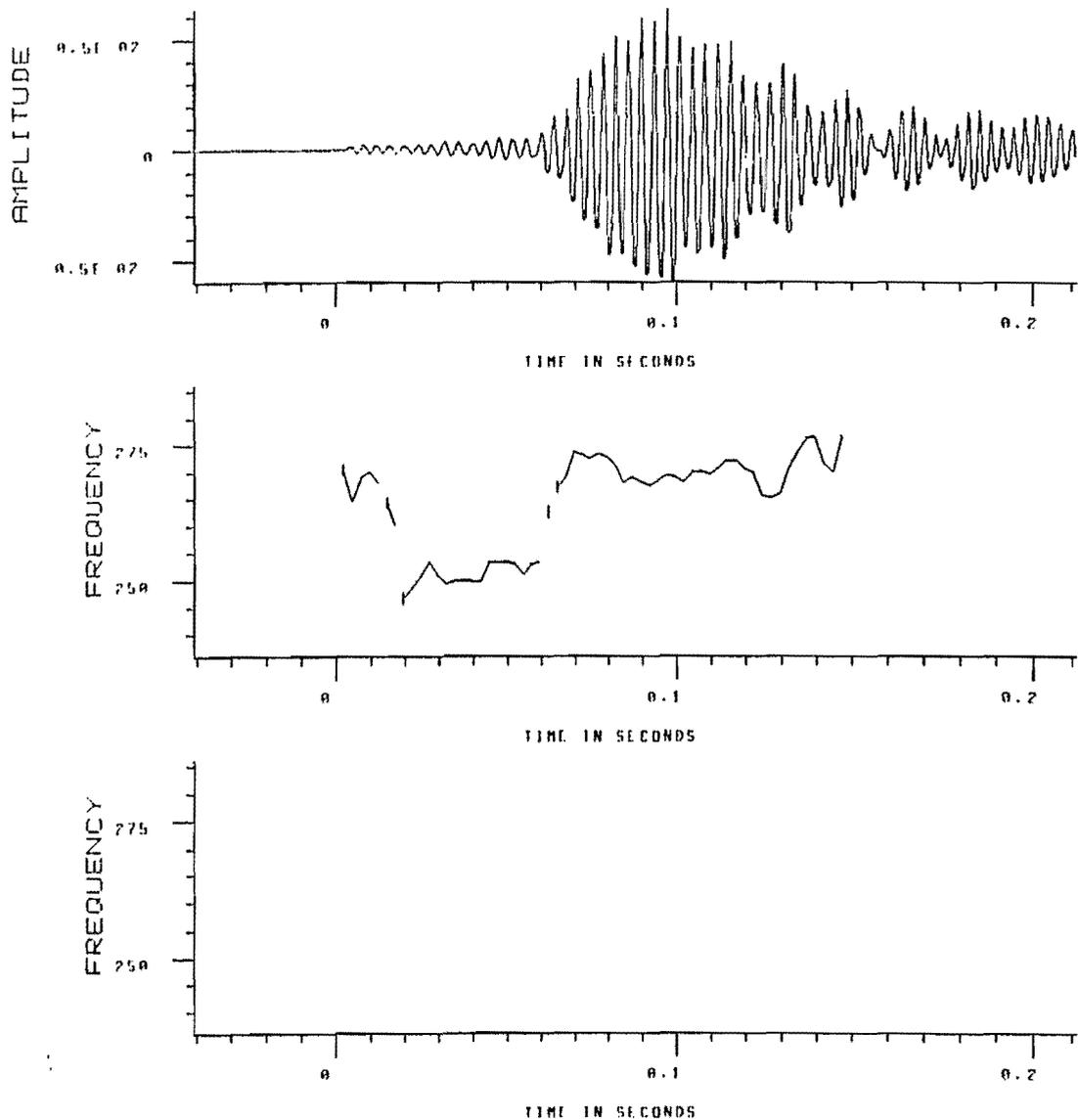
FIGURE 35. Here we see the results of applying a bandpass filter the center frequency of which does not correspond to any partial in the piece at that time. The filter, of course, passes in attenuated form the composite waveforms of the neighboring partials. The optimum-comb found some minima to track, as is shown in the center plot. Since the list of frequencies found by the optimum-comb is highly variable, it can be eliminated on this basis alone, as is shown in the lower plot.
