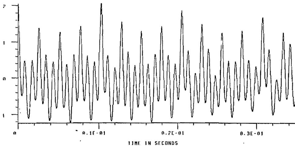
Figure 11. The autocorrelation of the waveform shown in figure 10. It has maxima at multiples of 98 Hz, representing the low G2 root note.
