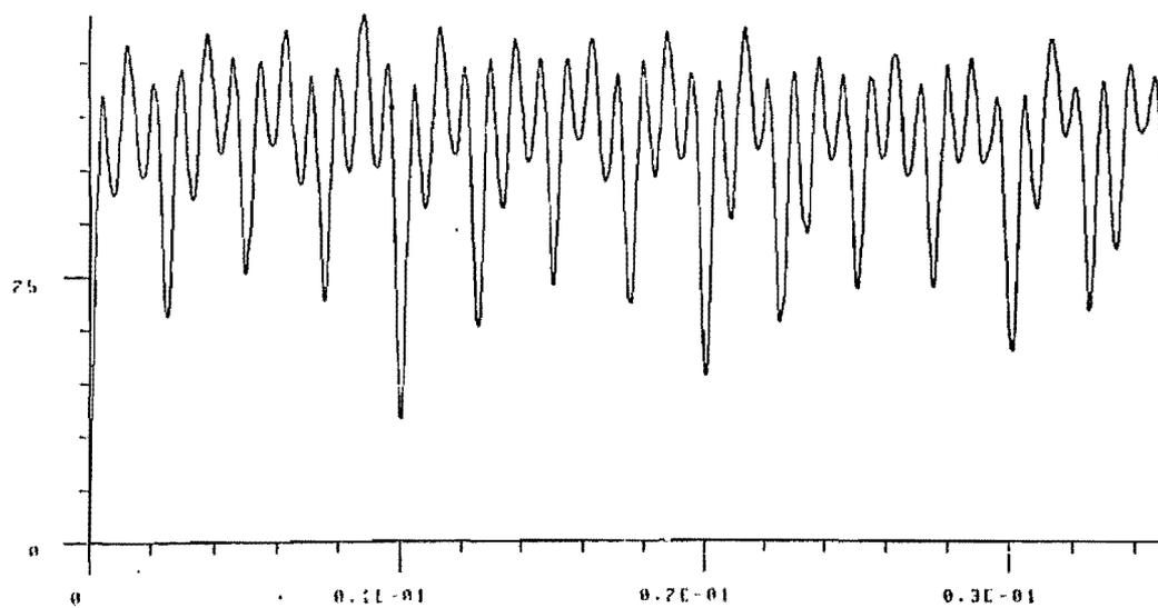
FIGURE 14. This is the results of applying the optimum-comb to the first chord of the brass choir in Tableaux D'une Exposition. The chord is a G-minor. The principal minima are subharmonics of G2 (about 98 Hz.).
