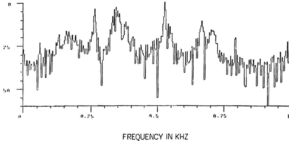
FIGURE 40. Discrete Fourier transform of a 4096 point (200 millisecond) segment of a piano duet. The time window is centered over the boundary between two notes. The lower voice persists throughout the window at a constant C4 (261.6 Hz). The upper voice is changing between an E4 (329.6 Hz) and an F4 (349.2 Hz). The region around the E4 and F4 is quite muddled with many peaks in evidence.
