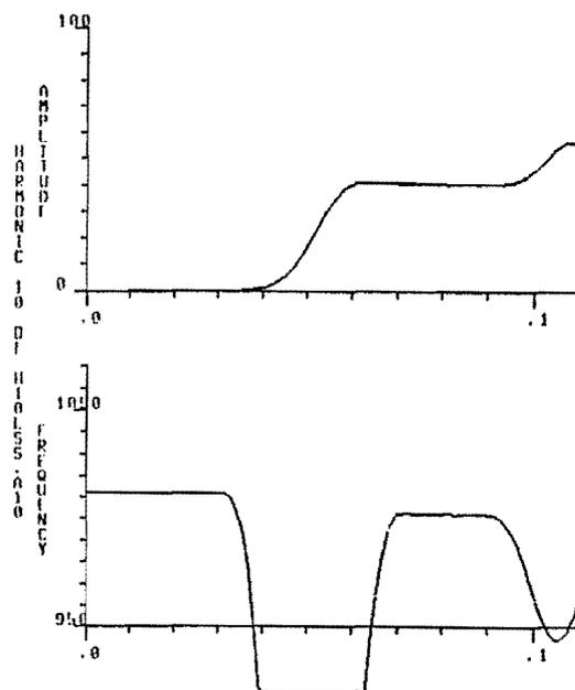
FIGURE A5. This shows the output of the heterodyne filter for a synthesized input signal which consists of a 100 Hz signal with a 10 millisecond linear attack on each harmonic. Each harmonic is 70% of the amplitude of the previous harmonic. The attack portion of the tone lasts only 1 period, which is extremely fast. The heterodyne filter cannot track the frequency during the attack portion and throughout some of the steady-state portion. The amplitude curves, however, are not grossly in error.
