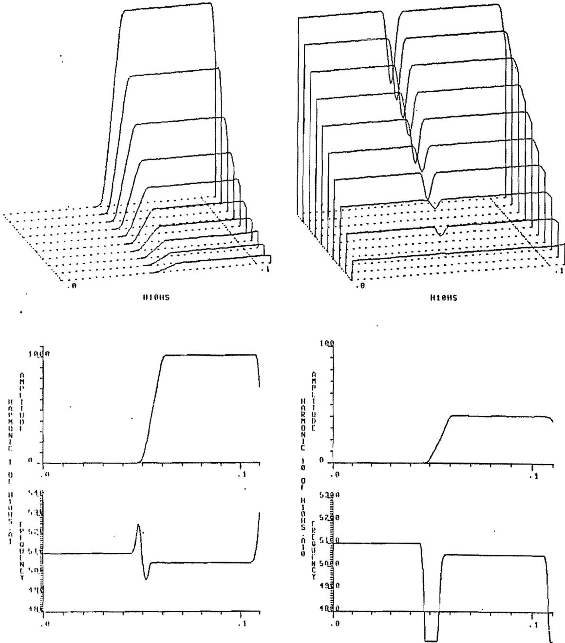
FIGURE A4. This shows the output of the heterodyne filter for a synthesized input signal which consists of a 505 Hz signal with a 10 millisecond linear attack on each harmonic. Each harmonic is 70% of the amplitude of the previous harmonic. The attack portion of the tone lasts only 5 periods, which is quite fast. As we would expect, the frequency trace for the first few periods is not accurate.
