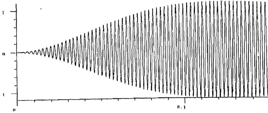
FIGURE 30. The response of a narrow bandpass filter to a pure sinusoid applied suddenly
