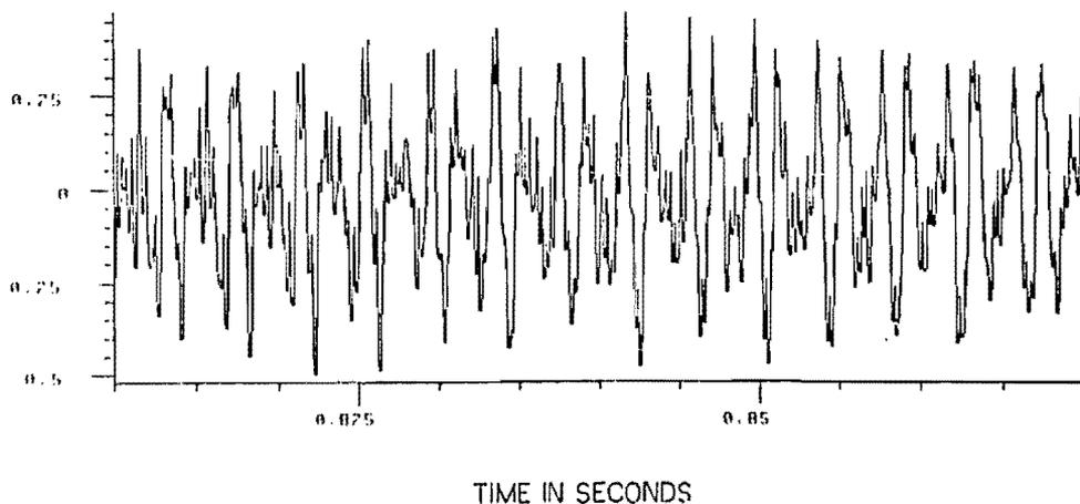
FIGURE 45. This is the waveform of a violin duet. One violin is playing a B4 (494 Hz) and the other is playing an F#4 (370 Hz). There is no periodicity evident to the unaided eye in the waveform.
