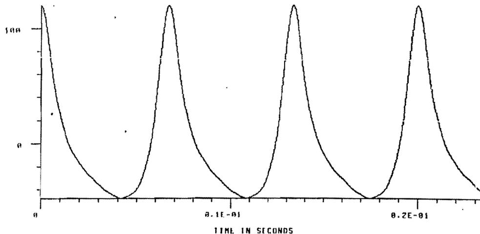
FIGURE 5. This is the autocorrelation of a periodic signal with 5 harmonics. As we see, the result is also periodic, although the harmonic amplitudes are entirely different from those of the input waveform.
