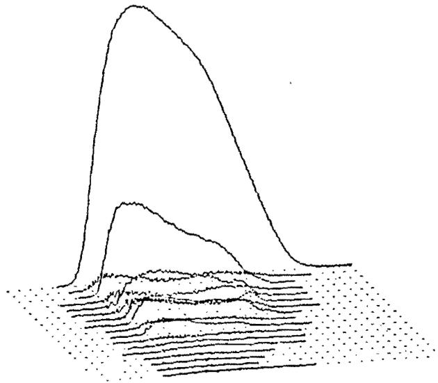
FIGURE 26. Perspective plot of analysis data from heterodyne filter, shown as an Amplitude x Frequency x Time perspective plot. The detailed frequency variation of each harmonic is not shown here. (X = time; Y = amplitude; Z = frequency, with the fundamental harmonic plotted in the background).
