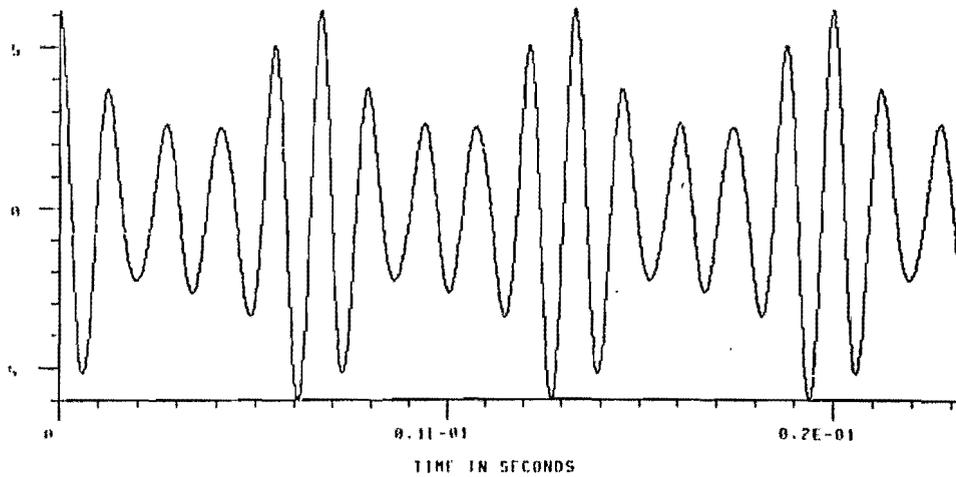
FIGURE 6. The autocorrelation of a periodic signal with only three harmonics: the 5th, 6th, and 7th. The autocorrelation is periodic with a period equal to the missing fundamental of the waveform.
