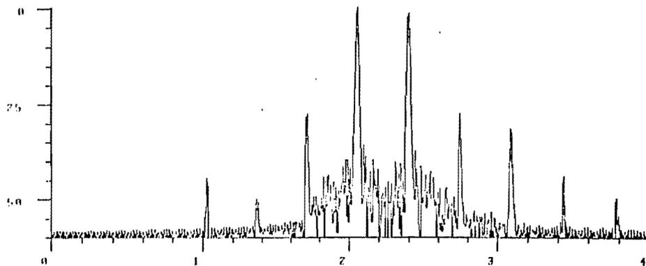
FIGURE 2. This is the discrete Fourier transform of the waveform in figure 1. As we can see, the first and second harmonics are entirely absent. Despite their absence, the waveform in figure 1 is quite periodic.
