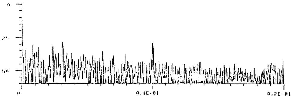
FIGURE 37. This is the cepstrum of a segment of the waveform of a brass choir. The waveform was taken from the first brass chord of Ravel's orchestration of *Mussorgsky's Tableaux D'une Exposition*. The cepstrum does not seem to produce a distinct peak corresponding to any periodicity in the input signal in this polyphonic case.
