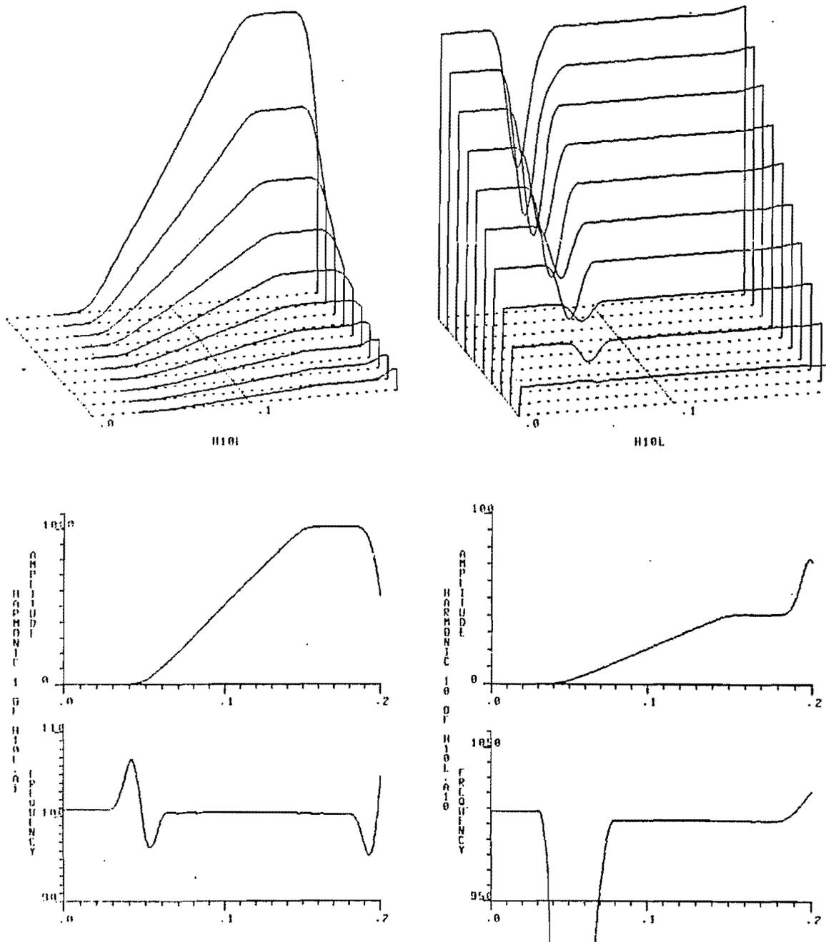
FIGURE A2. This shows the output of the heterodyne filter for a synthesized input signal which consists of a 100 Hz signal with a 100 millisecond linear attack on each harmonic. Each harmonic is 70% of the amplitude of the previous harmonic.
