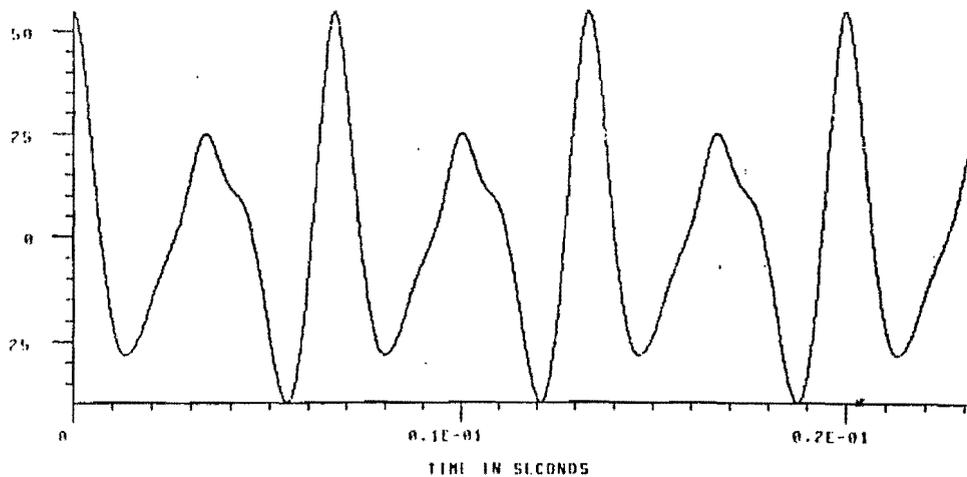
FIGURE 7. The autocorrelation of a periodic signal with only harmonics 2, 3, 4, 6, 8, 9, and 10 present. This is what would occur, for instance, if two tones at 300 Hz and 450 Hz were present simultaneously. This represents the musical interval of the perfect fifth. Any two tones at this interval will produce a periodicity in the autocorrelation equal to an implied fundamental period of the composite waveform.
