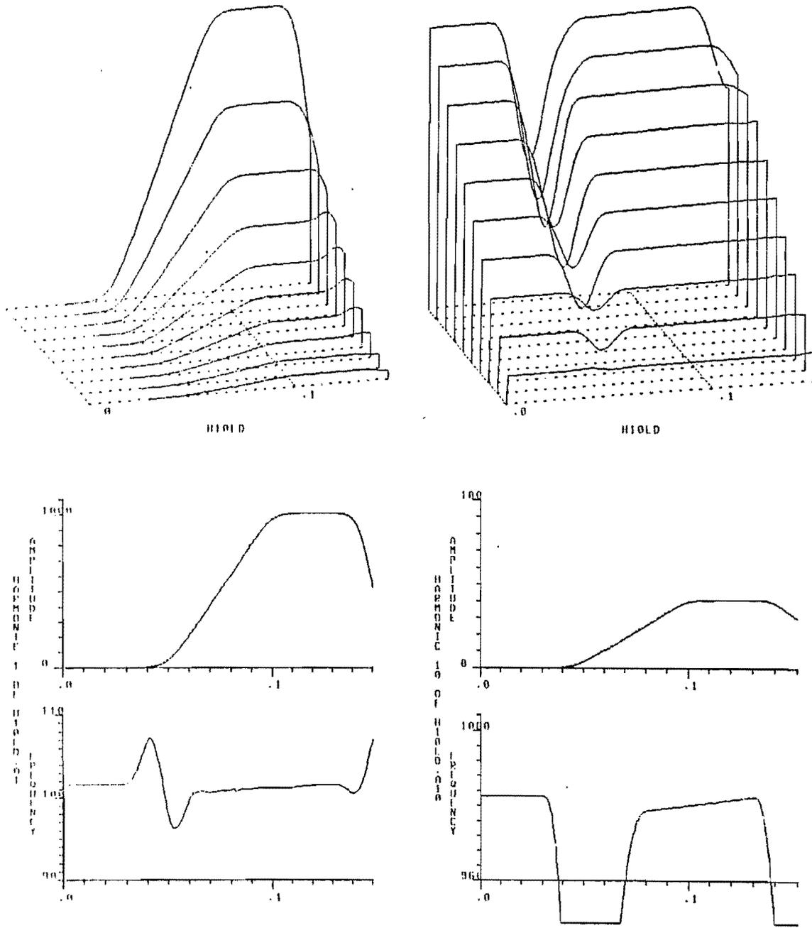
FIGURE A8. This shows the output of the heterodyne filter for a synthesized input signal which consists of a 100 Hz signal with a 50 millisecond linear attack on each harmonic. Each harmonic is 70% of the amplitude of the previous harmonic. Here we slew the frequency of the note from 100 Hz to 101 Hz over the duration of the tone. This is a 1% change, less than a quarter-step. As in the previous figure, the heterodyne filter seems to track acceptably.
