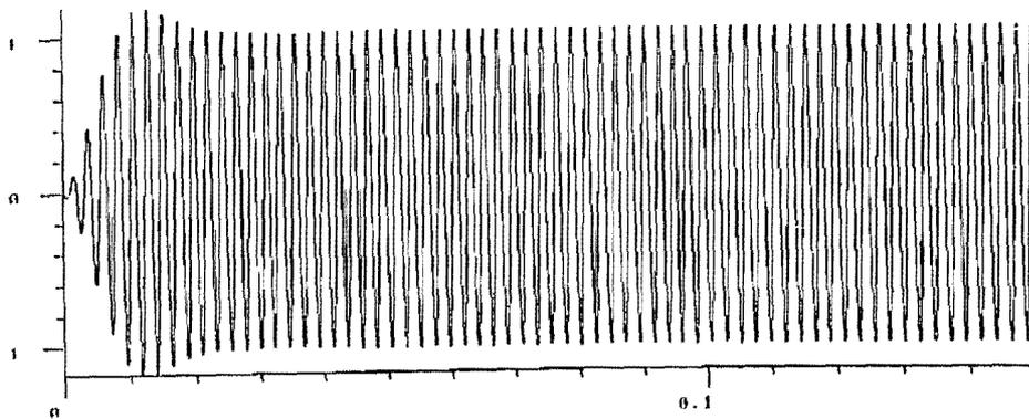
FIGURE 31. The response of a broad bandpass filter to a pure sinusoid applied suddenly.
