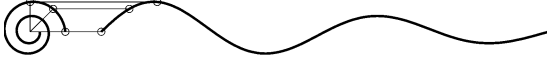
Fig. 1. Damped oscillator in state space form. Left: At each time step, the state vector s rotates by \omega and its length becomes shorter. Right: The actual waveform is a one dimensional projection from the two dimensional state vector. The stochastic model assumes that there are two independent additive noise components that corrupt the state vector s and the sample y , so the resulting waveform y_{1:T} is a damped sinusoid with both phase and amplitude noise.
