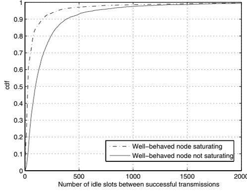
Fig. 3: The cdf of the number of idle slots between successful transmission for a saturating and non-saturating legitimate terminals.
