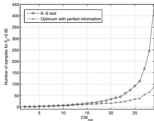
Fig. 9: Number of samples needed to detect a misbehaving terminal using IEEE 802.11 DCF with different  $CW_{\min}$  and with  $P_D = 0.95$ .
