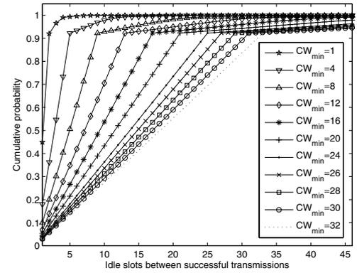
Fig. 7: Cdf of the number of idle slots between successful transmissions when a misbehaving terminal uses IEEE 802.11 DCF with different  $CW_{\min}$ .
