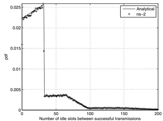
Fig. 2: The pdf of the number of idle slots between successful transmissions for an IEEE 802.11 DCF network with 10 nodes.
