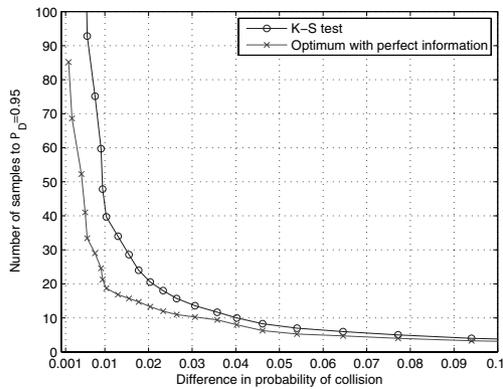
Fig. 10: Number of samples needed to detect a shift in collision probability with  $P_D = 0.95$ .
