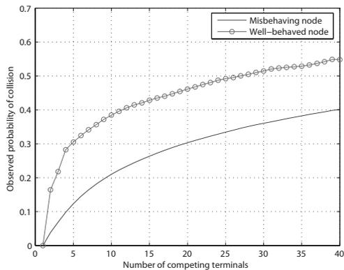
Fig. 1: Effect of having just one misbehaving node in the observed probability of collision of an IEEE 802.11 DCF network.
