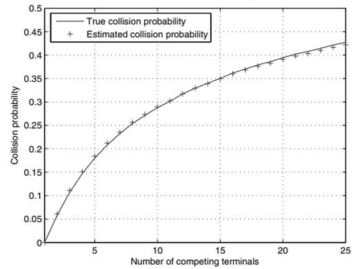
Fig. 5: Estimated collision probability using the collision factor for  $U = 15$ .
