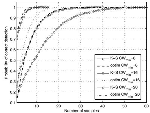
Fig. 8: Performance of the K-S detector vs. optimum detector when a misbehaving terminal uses IEEE 802.11 DCF with different  $CW_{\min}$ .
