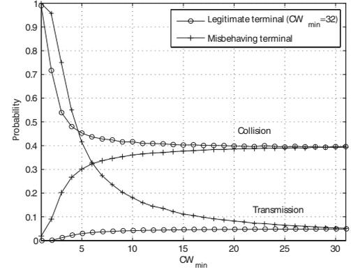
Fig. 6: Probability of transmission and collision when a misbehaving terminal uses IEEE 802.11 DCF with different  $CW_{\min}$ .
