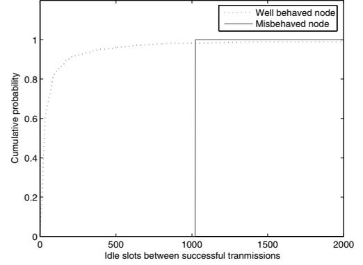
Fig. 4: Example of a misbehaving terminal with transmission probability lower than that of a legitimate terminal.
