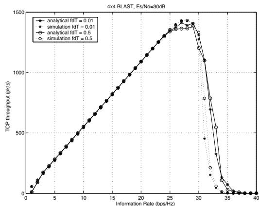
Fig. 2. TCP throughput for analytical and simulation results.
