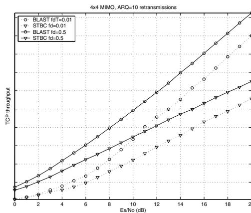
Fig. 4. Maximum TCP throughput for BLAST and STBC vs. Doppler.
