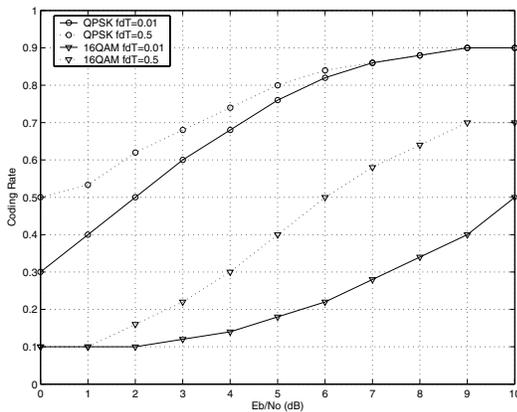
Fig. 5. Optimal coding rate for TCP over  $2 \times 2$  BLAST.
