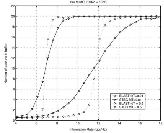
Fig. 6. Comparison of buffer occupancy for  $4 \times 4$  BLAST and STBC for different Doppler values. Buffer is 20 packets and  $E_s/N_o = 10$  dB.
