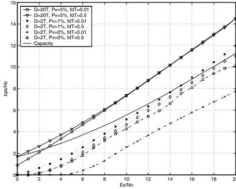
Fig. 7. Rate that maximizes the video throughput for  $2 \times 2$  BLAST under different delay and error constraints.
