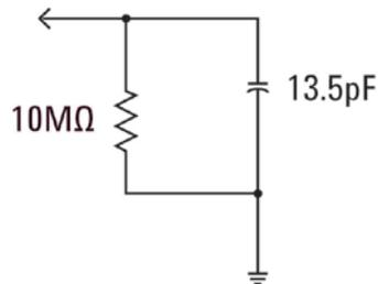
**Figure 24** 10:1 passive probe and scope loading model
