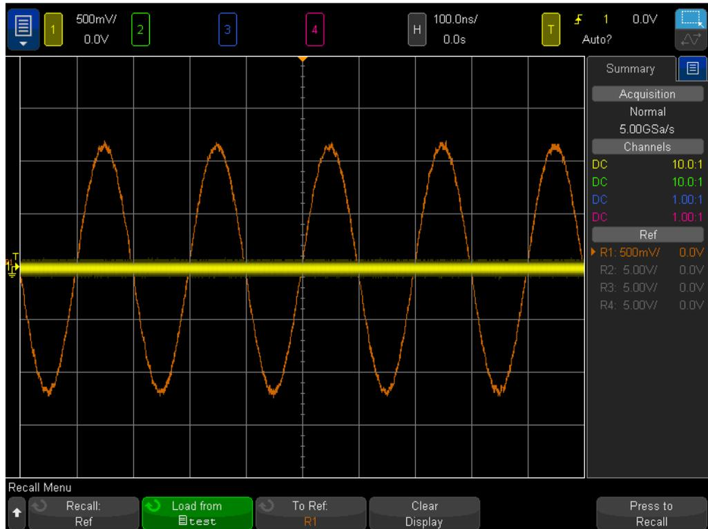
Figure 20 Recalling the scope's setup configuration and waveform
