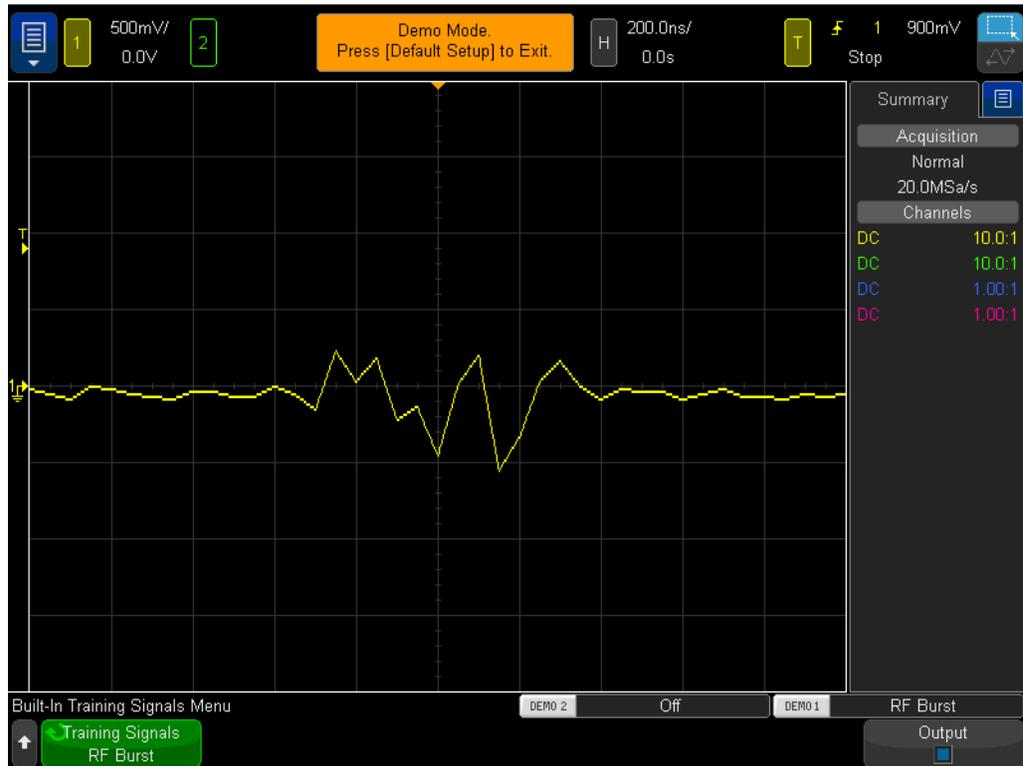
**Figure 48** Zooming in reveals an under-sampled waveform
