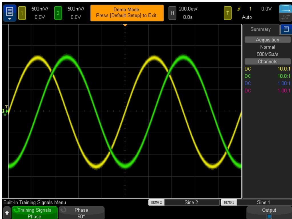
**Figure 39** Performing measurements on phase delayed signals
