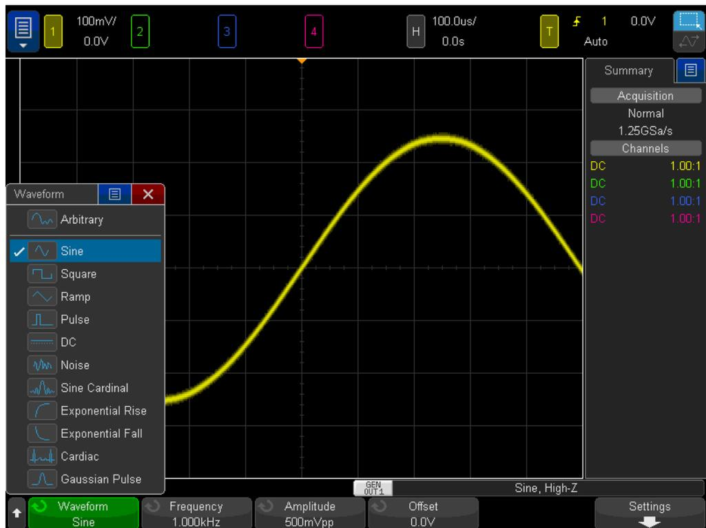
**Figure 25** Using the scope's built-in WaveGen function generator
