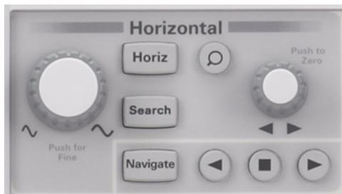
**Figure 4** Oscilloscope horizontal (X-axis) controls
