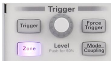
**Figure 6** Oscilloscope trigger level control
