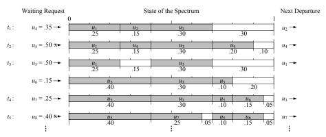
Figure 2: An example of the admission and departure processes and the resulting spectrum fragmentation.
