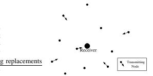
Fig. 1. Nodes distributed in a plane and a single receiver with a multipacket reception capability. Five nodes transmit simultaneously. The high power signal from the nearby node results in failure of the 4 transmissions from the distant nodes. Due to the multipacket reception capability, if the nearby node does not transmit, these 4 transmissions can be captured.
