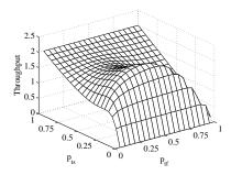
Fig. 7. The overall throughput (S) under the GDP protocol in a fading-free environment. The nodes are distributed according to the rings model with  $r_1=1, r_2=2, n_1=2$ , and  $n_2=10$ .
