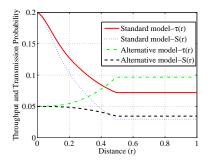
Fig. 4. The transmission probability  $(\tau(r))$  and the throughput (S(r)) as a function of distance under the GDP protocol using the Standard Model  $(p_{\rm ts}=0.2,\,p_{\rm tf}=0.05)$  and the Alternative Model  $(p_{\rm ts}=0.05,\,p_{\rm tf}=0.2)$ . The system operates according to the vulnerability circle model with  $\alpha=2$  and Uniform distribution of 12 nodes in a disk of radius 1.
