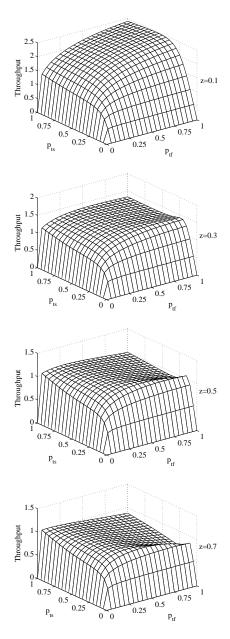
Fig. 14. The throughput (S) under the GDP protocol in a system with fading. 10 nodes are distributed according to the disk model with z=0.1, z=0.3, z=0.5, and z=0.7.
