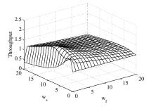
Fig. 10. The throughput (S) under the GDCW protocol in a fading-free environment. The nodes are distributed according to the rings model with  $r_1 = 1, r_2 = 2, r_3 = 3, n_1 = 1, n_2 = 3$ , and  $n_3 = 9$ .
