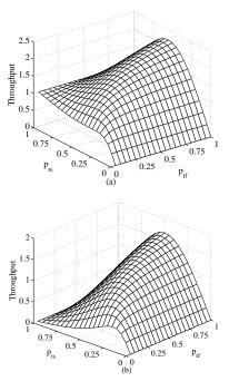
Fig. 6. (a) The overall throughput (S) and (b) the throughput of the distant nodes. The system operates under the GDP protocols in a fading-free environment and the nodes are distributed according to the rings model with  $r_1=1, r_2=2, n_1=1$ , and  $n_2=5$ .
