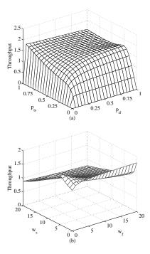
Fig. 12. The throughput (S) under (a) the GDP protocol and (b) the GDCW protocol in a fading-free environment. 10 nodes are distributed according to the disk model.
