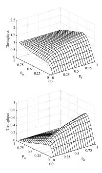
Fig. 8. (a) The overall throughput (S) and (b) the throughput of the nodes at  $r_3$ , under the GDP protocol in a fading-free environment. The nodes are distributed according to the rings model with  $r_1 = 1, r_2 = 2, r_3 = 4, n_1 = 1, n_2 = 2$ , and  $n_3 = 4$ .
