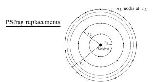
Fig. 2. Nodes deployed according to the rings model on rings whose radii are  $r_1, r_2, \ldots, r_L$ .
