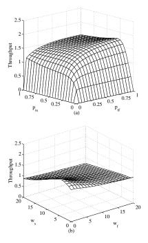
Fig. 13. The throughput (S) under (a) the GDP protocol and (b) the GDCW protocol in a system with fading. 10 nodes are distributed according to the disk model.
