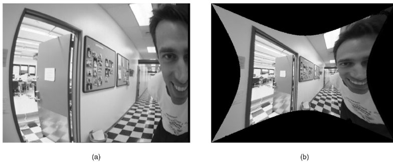
Fig. 5. (c) Image produced by a Computar 2.5mm lens and a Computar 1/3" CCD board camera. (b) Distortion parameters recovered via the minimization of \xi_3 are used to map (a) to perspective image. Notice that straight lines in the scene, such as door edges, map to straight lines in the undistorted images.
