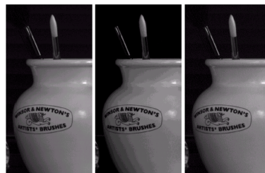
a b c FIGURE 8.4 (a) Original image (b) Uniform quantization to 16 levels (c) JGS quantization to 16 levels
