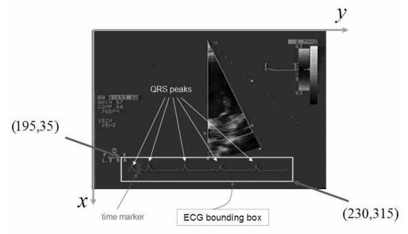
1- [10 pts.] Take the first image in the sequence, extract the box including the ECG and segment the image into foreground (ECG signal) and background. The coordinates of the opposite corners of the box are given in the above figure. For
