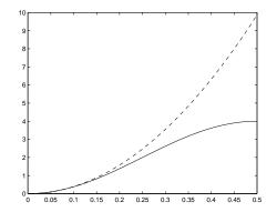
In the figure there is |H(u,0)| in discrete and continuous case. Solid line: discrete case, i.e.  $|H(u,0)| = 2 - 2\cos(2\pi u)$ . Dotted line: continuous case, i.e.  $|H(u,0)| = (2\pi)^2 u^2$ .
