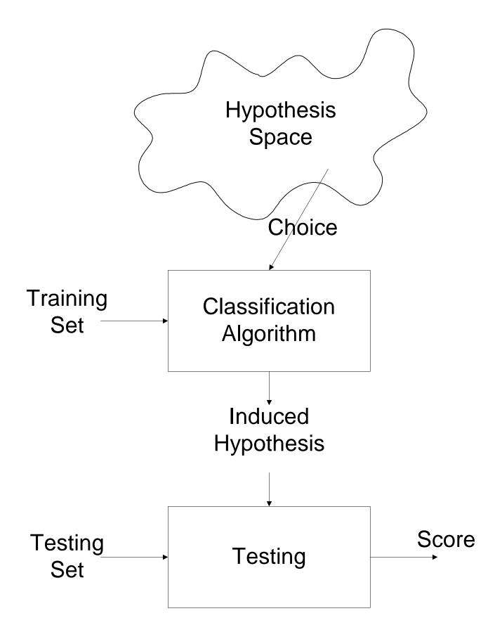
Block Diagram of a Classification Algorithm
