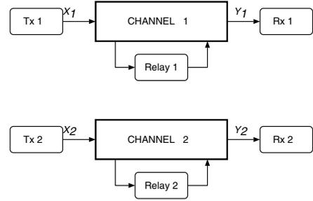
Fig. 3. Dedicated relays for orthogonal multiuser channels
