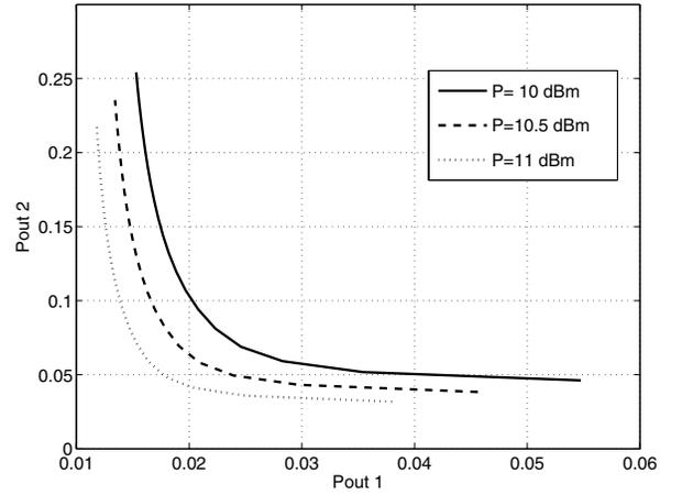
Fig. 7. Outage probabilities, unequal transmit powers
