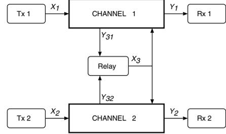
Fig. 4. Broadcast relay for orthogonal multiuser system
