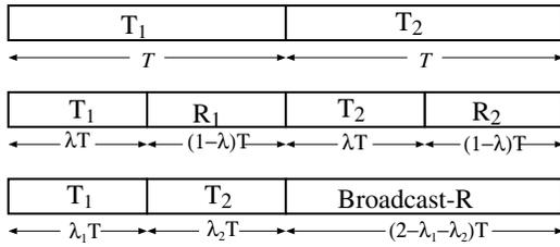
Fig. 2. Three transmission schemes: Non-Relay Dedicated Relay, Joint Relay
