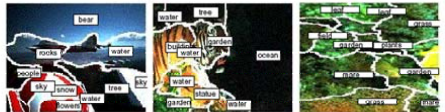
Fig. 9. Some test results which are not satisfactory. Words that are wrongly predicted are the ones with very low recall values. The problem mostly seen in the third image is since green blobs occur mostly with grass, plants or leaf rather than the under water plants.
