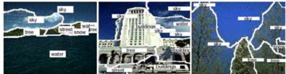
Fig. 8. Some examples of the labelling results. The words overlaid on the images are the words predicted with top probability for corresponding blob. We are very successful in predicting words like sky, tree and grass which have high recall. Sometimes, the words are correct but not in the right place like tree and buildings in the center image.
