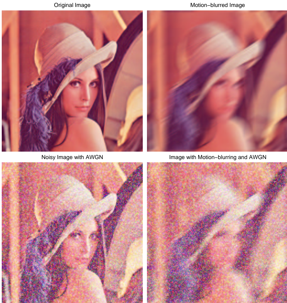
Figure 1: “Lena.jpg” in different conditions: the original image; the motion-blurred image; the noisy image with AWGN ( \sigma_n = 0.5 ); the motion-blurred image with AWGN ( \sigma_n = 0.5 ).
