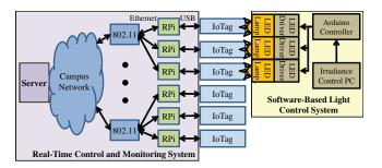
Figure 2: A schematic diagram of the envisioned IoTag testbed.
