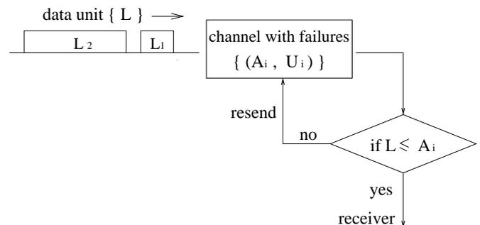
Fig. 1. Packets sent over channels with failures
