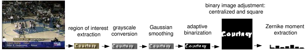
Fig. 3. Processing steps for Zernike moment extraction.
