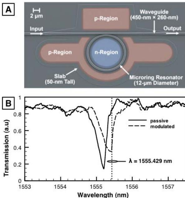
**Fig. 1** **a)** Scanning-electron-microscope (SEM) image of the microring modulator. N and P doping are indicated in the interior and exterior of the microring, respectively. **b)** Wavelength spectrum of the microring in its passive and modulated states. The wavelength of the modulated signal is indicated by a vertical dashed line.
