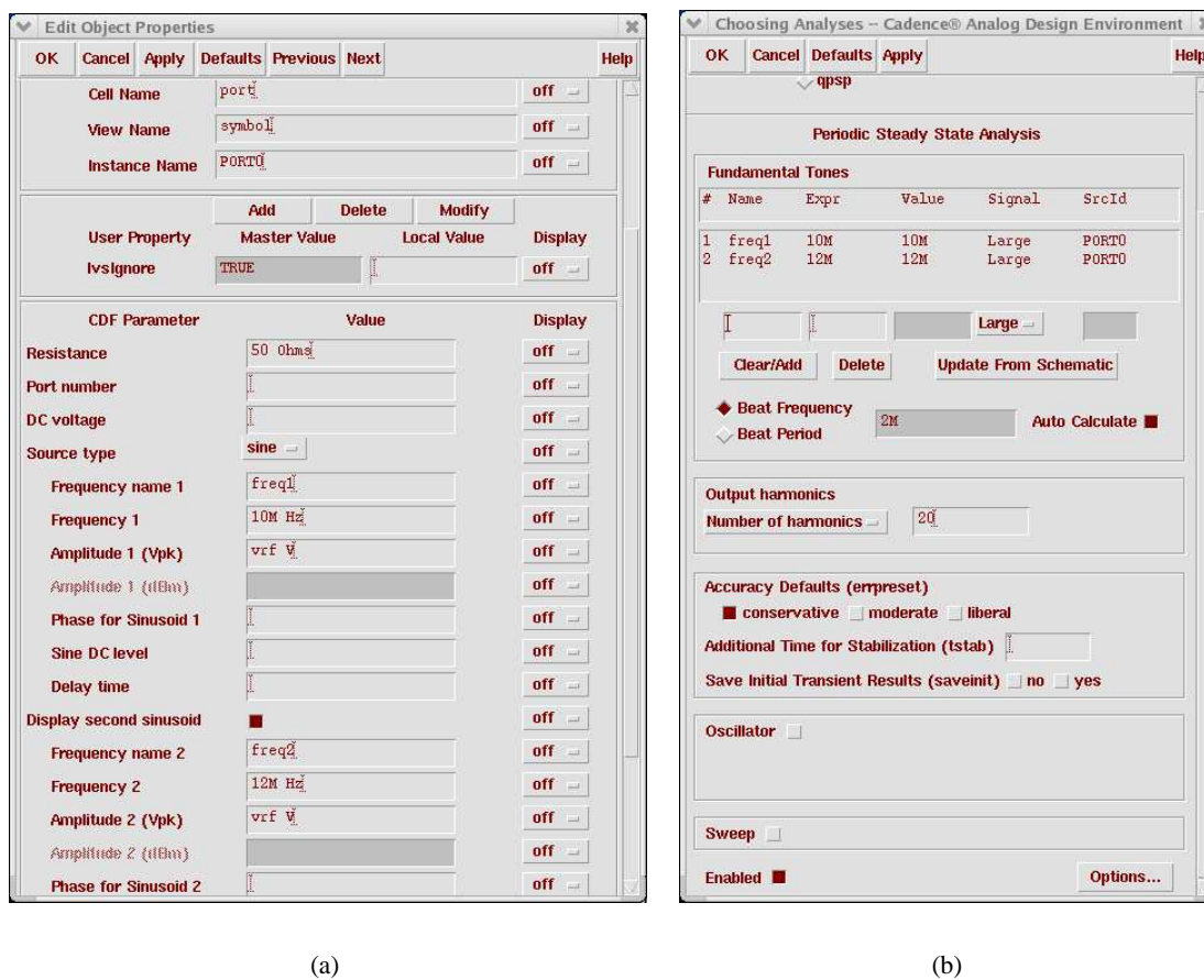
Fig. 2. (a) Properties of the port used in the test setup of fig. 1(a) (b) PSS analysis form.
