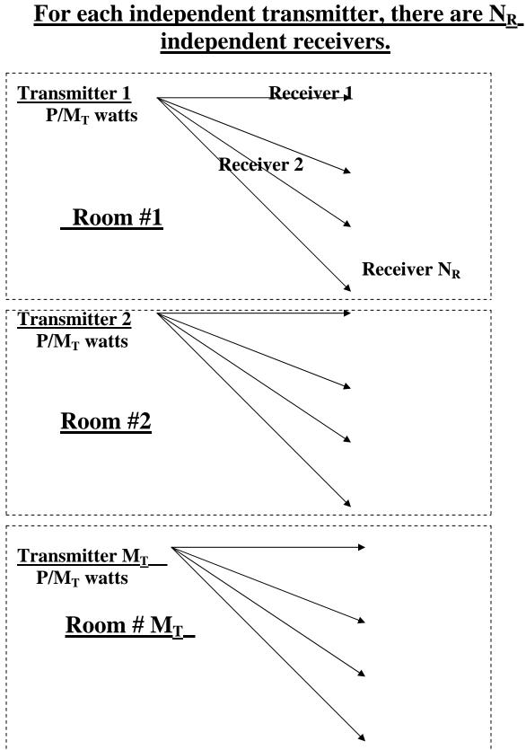
In <u>each individual room</u>, we are transmitting  $P/M_T$  watts and using  $N_R$  receivers so the capacity in each individual room would be
