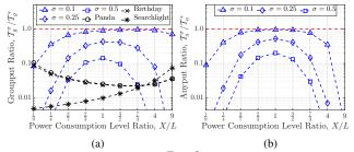
Fig. 3: Throughput performance of EconCast when operating in: (a) groupput mode and (b) anyput mode, with N=5,  $\rho=10\,\mu\mathrm{W}$ ,  $L+X=1\,\mathrm{mW}$ , and  $\sigma\in\{0.1,0.25,0.5\}$ , as a function of X/L.
