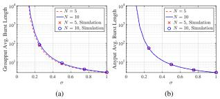
Fig. 4: Analytical (curves) and simulated (markers) average burst length of EconCast when operating in: (a) groupput mode and (b) anyput mode, with  $N \in \{5, 10\}$ ,  $\sigma \in \{0.25, 0.5\}$ ,  $\rho = 10 \, \mu \text{W}$ , and  $L = X = 500 \, \mu \text{W}$ .
