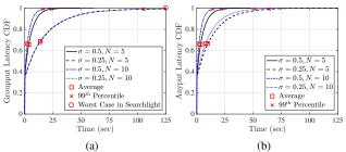
Fig. 5: The CDF, mean, and  $99^{\rm th}$  percentile latency of EconCast when operating in: (a) groupput mode and (b) anyput mode, with  $N\in\{5,10\},$   $\sigma\in\{0.25,0.5\},$   $\rho=10\,\mu{\rm W},$  and  $L=X=500\,\mu{\rm W}.$
