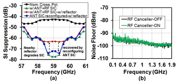
Fig. 7. (a) Measured SI suppression across frequency with antenna and RF cancellation configured. Bringing a reflector 1.5cm away from the antennas degrades the SI suppression, but it can be recovered by reconfiguring the antenna cancellation. (b) RF canceller's effect on the receiver output noise (RBW=51kHz).
