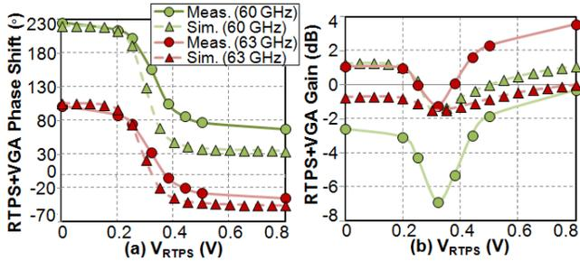
Fig. 6. Measured and simulated (a) phase shift and (b) gain of the RTPS-VGA test structure with VGA on maximum gain setting.
