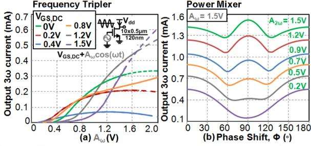
Fig. 2. Third harmonic current (a) as a function of fundamental amplitude and gate bias voltage in a conventional frequency tripler for a  $\frac{10 \times 0.5 \mu\text{m}}{120\text{nm}}$  device. (b) as a function of second-harmonic amplitude  $A_{2\omega}$  and relative phase  $\phi$  between the fundamental and second-harmonic drive in  $\frac{10 \times 0.5 \mu\text{m}}{120\text{nm}}$  power mixer.  $A_{\omega}=1.5\text{V}$
