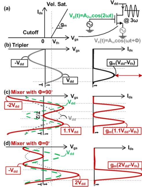
Fig. 3. (a) Power mixer configuration and piece-wise linear current model. (b) Maximum fundamental gate drive and device current in a tripler biased at 0V. Gate-source voltage and current in a power mixer for  $A_{2\omega}=A_{\omega}=1.5\text{V}$  and (c)  $\phi = 90^\circ$ , (d)  $\phi = 0^\circ$ .
