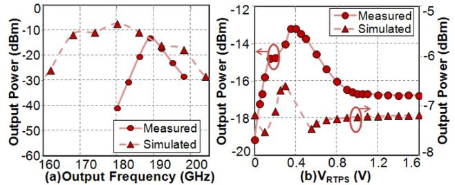
Fig. 7. (a) Saturated output power across output frequency.  $P_{in,meas.} = 11\text{dBm}$  and  $P_{in,sim.} = 7\text{dBm}$ . VGA is at maximum gain,  $V_{RTPS}=0.3\text{V}$  (optimal). (b) Variation in output power at 189GHz with  $V_{RTPS}$ . Simulations are at nominal value of 180GHz.
