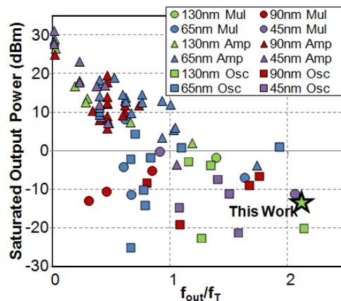
Fig. 1. Comparison of our work with state-of-the-art CMOS signal sources across output frequency normalized to technology  $f_T$ .
