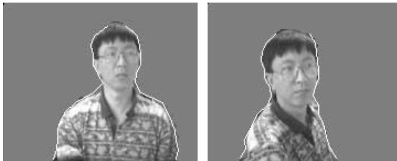
Figure 2-7: Comparison of the limits of shape analysis for blob tracking. In the left image, the shape feature is strong and the head region and the shoulder regions can be easily separated based on the foreground shape information. But in the right image, the shape feature is not so obvious and shape analysis is sensitive to noise.
