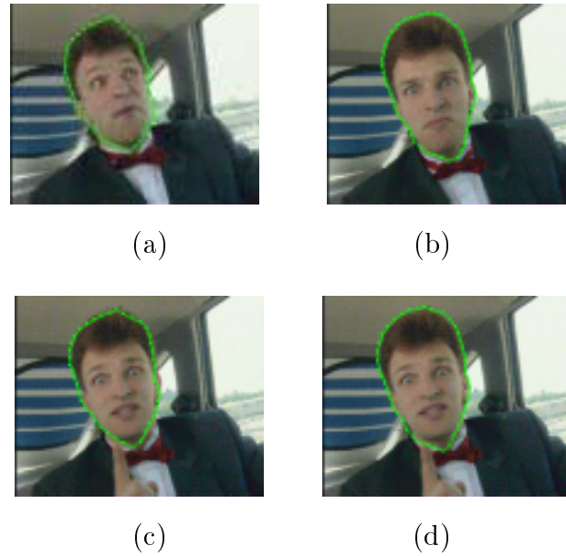
Figure 5-5: Illustration of the necessity of bi-directional tracking and result merging. (a), (b) are the user defined VO on the 118th and the 132nd frame of the Carphone sequence. (c) is the tracked object contour on the 125th frame by forward tracking. (d) is the tracked object contour on the 125th frame by backward tracking.
