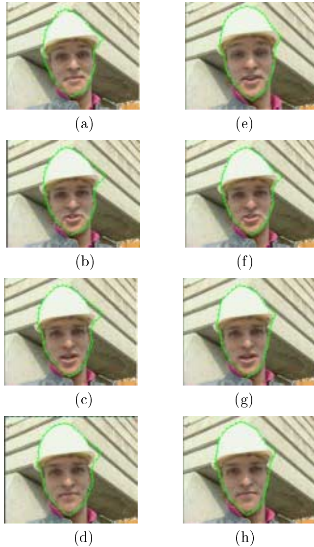
Figure 5-9: An example of iterative interpolation on the Foreman sequence. In the first round, the user specifies C_b at frame 50 and C_e at frame 100, the global search parameters are height = 15 (pixels), width = 4 (pixels). (a) to (e) are results on frames 80, 84, 87, 90, 94 at this round. In the second round, previous contour result on frame 80 is used as C_b and contour result on frame 94 is used as C_e , the global search parameters are reduced to be height = 4 , width = 4 . The new interpolation results on frame 84, 87, 90 are showed in (f), (g), (h), respectively.
