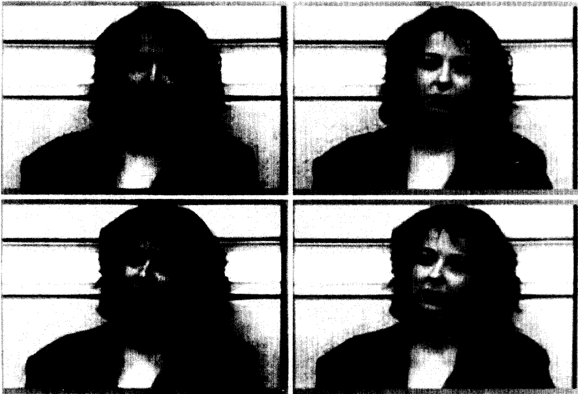
Fig. 13. Stills from sequence 'jelena' (frames 210 and 408) coded with p \times 64 at 48 kbps, respectively, without (left) and with (right), model-assisted rate control.
