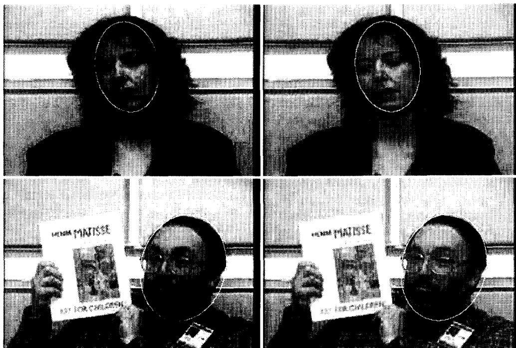
Fig. 10. Stills from sequences 'jelena' and 'jim' coded with 3D SBC at 96 kbps, respectively without (left), and with (right), model-assisted DBA, with the face location models in white obtained manually.
