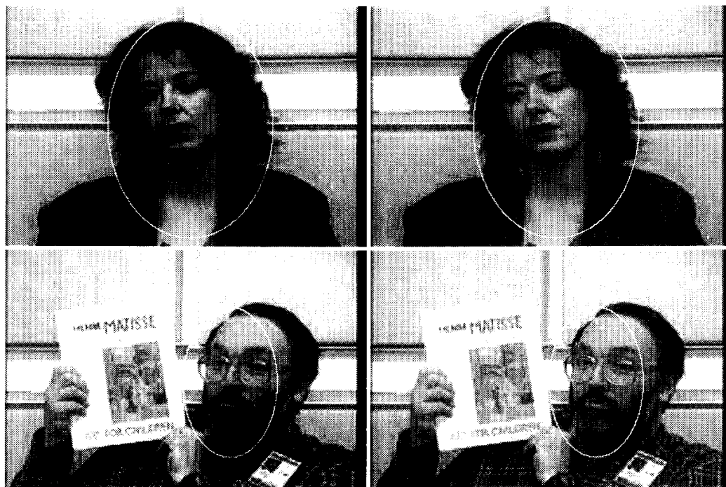
Fig. 14. Stills from sequences 'jelena' and 'jim', coded with 3D SBC at 96 kbps, respectively without (left), and with (right), model-assisted DBA, with face locations models in white obtained by automatic detection algorithm.
