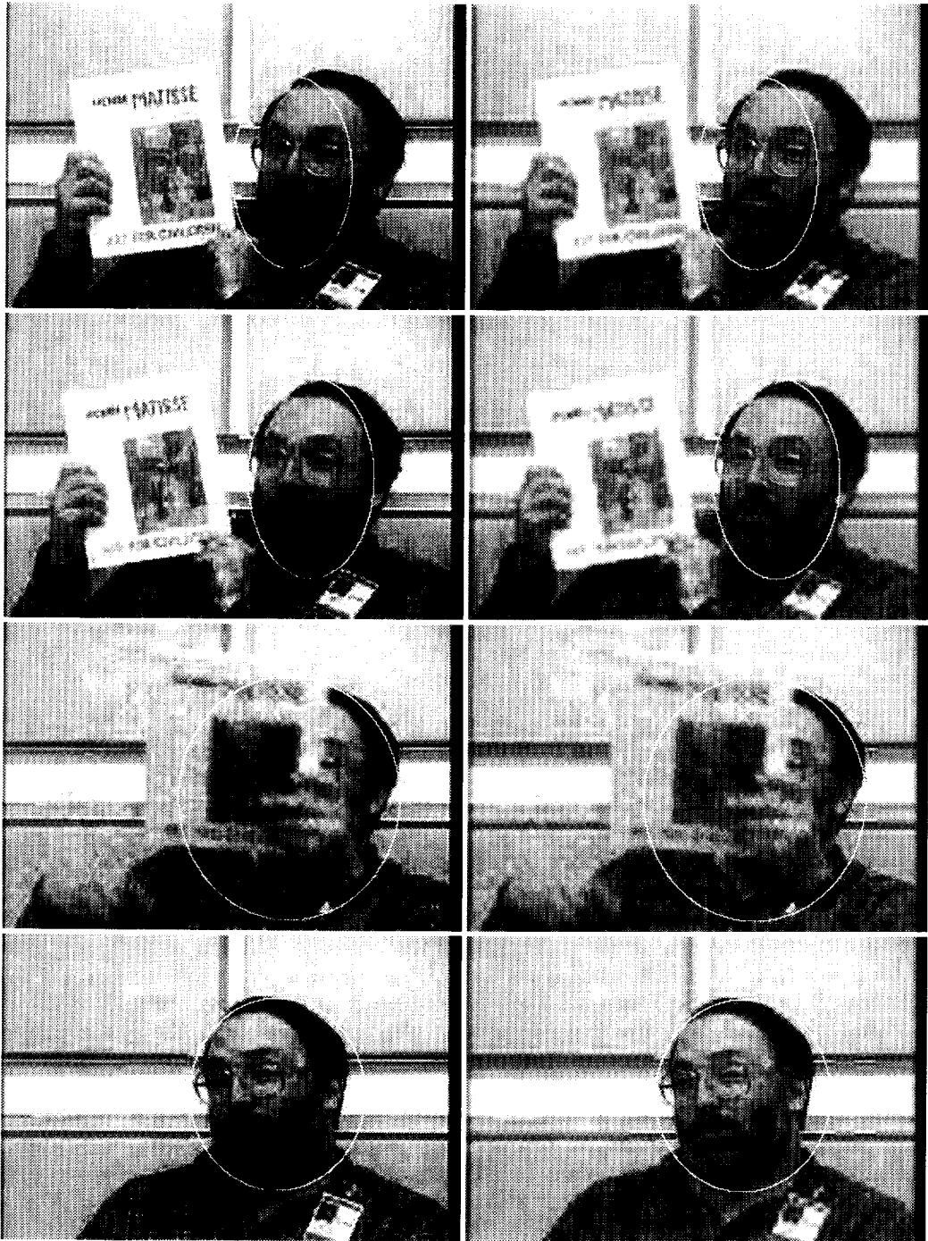
Fig. 15. Stills from sequence 'jim' coded with 3D SBC at 96 kbps with model-assisted DBA, with different amounts of bit transfer to facial area. The average bit transfer is 10% and 15% of the total bit-rate for the stills on the left and right, respectively.
