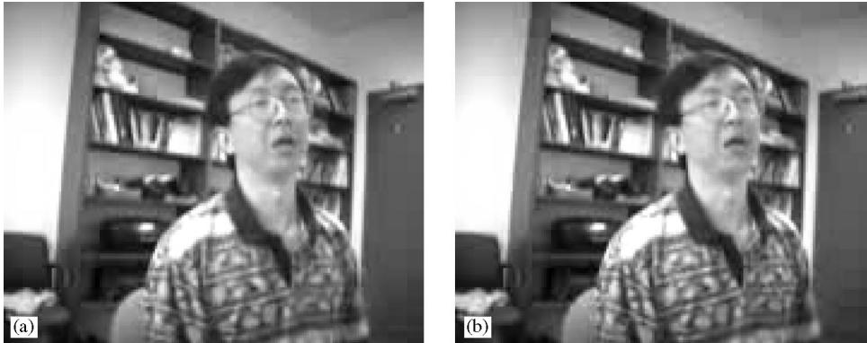
Fig. 17. Comparison of a typical pair of reconstructed frames. (a) The reconstructed 260th frame (of the testing sequence) with Scheme 1; (b) the reconstructed 260th frame with *tmn-2.0*. The facial region of the left image (a) is clearer than that of the right image (b).
