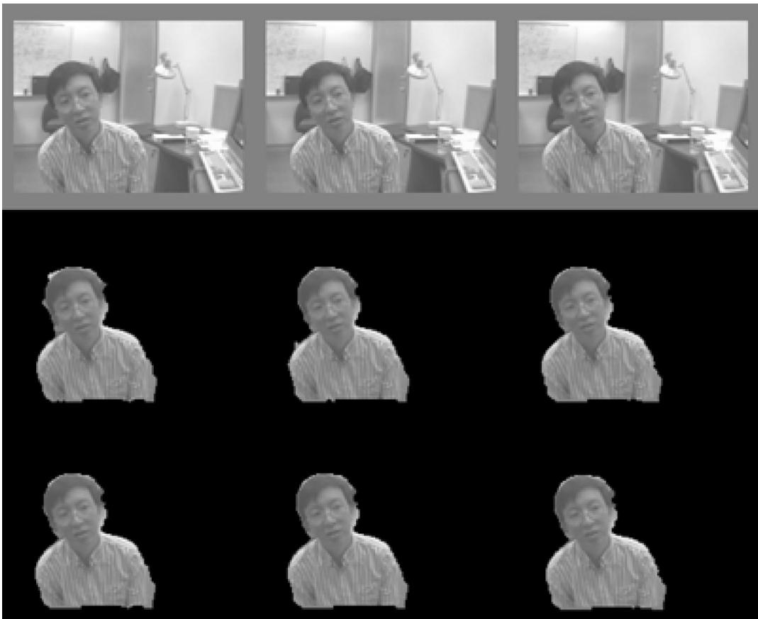
Fig. 10. Comparison of filter effects. The first row from left to right is three consecutive original frames. The second row is their segmented result without spatial/temporal filtering and the third row is the final result with spatial/temporal filtering. We can see that the temporal high-frequency noise on the boundary is effectively removed.
