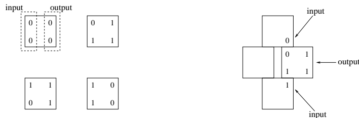
Fig. 1. Since a tile glues to other tiles only if their corner labels match, operation 0 \oplus 1 = 1 is performed. The correct output tile simply attaches itself to the preassembled input tiles, effectively yielding the output bit.
