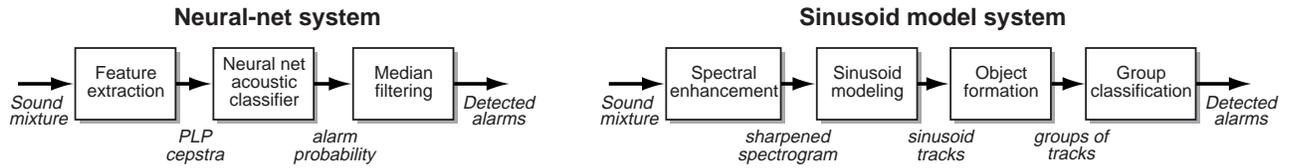
**Figure 2:** Block diagrams of the two alarm detection systems. Left: baseline system, adapted from a connectionist speech recognizer. Right: Sinusoid model based system.
