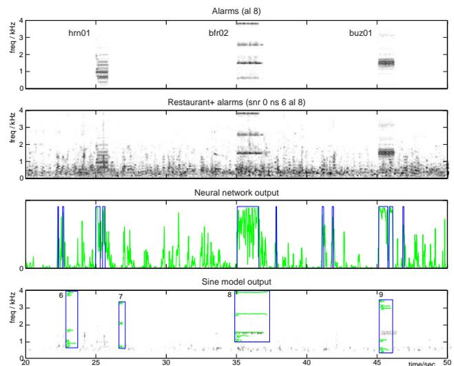
**Figure 4:** Comparison of systems’ performances. Three alarm sounds (top panel) are mixed with the restaurant babble giving the second panel. The filtered alarm probability from the neural network is shown in panel 3 (showing multiple false alarms due to the mismatch between training and test background noise). The bottom panel shows the alarm groups located by the sinusoid modeling system (which fails to detect the horn because it is inconsistent with the hand-defined ‘alarm-like’ criteria).
