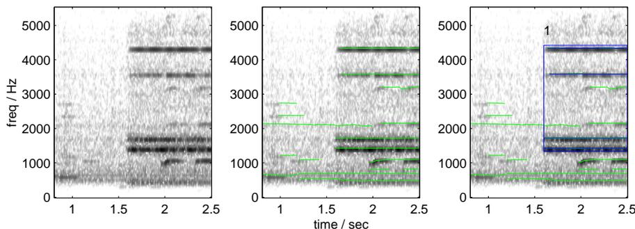
**Figure 3:** Stages in the sinusoid modeling system. The spectrogram on the left shows the strong horizontal energy components indicating an alarm sound. In the middle panel, the extracted sinusoid tracks are overlaid, finding both alarm and background components. Track group properties allow correct identification of the alarm energy in the third panel.
