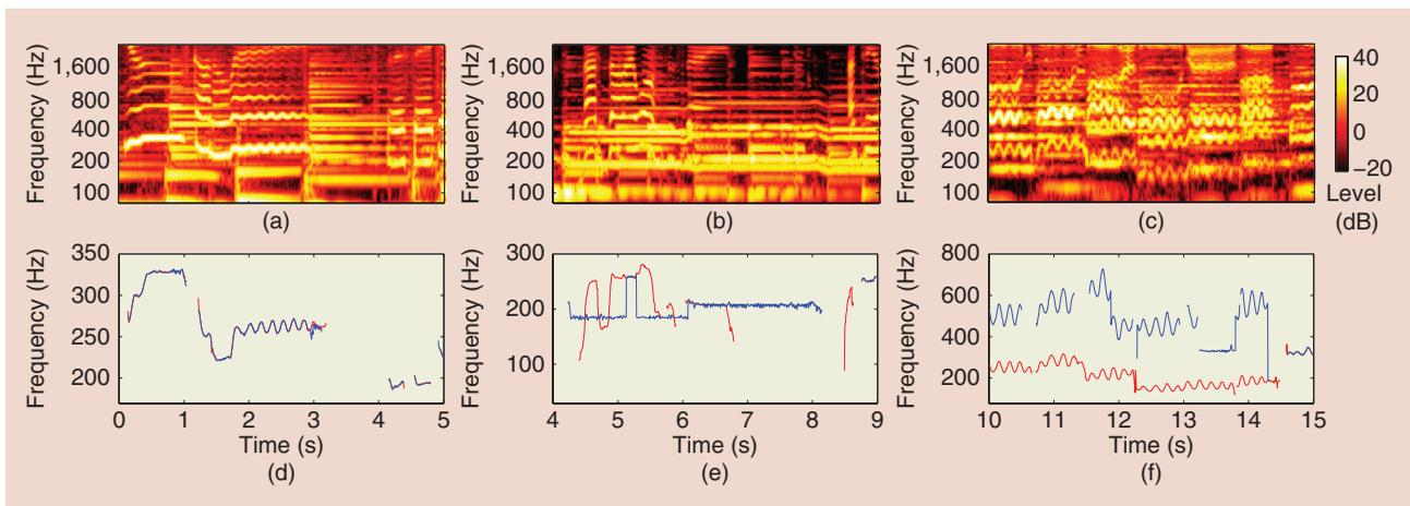
**[FIG2]** Case study examples: (a)–(c) show the log-frequency spectrogram of three excerpts in the genres of (a) vocal jazz, (b) pop, and (c) opera. Parts (d)–(f) show the extracted melody [16] (blue) and ground truth (red) for each excerpt, respectively.
